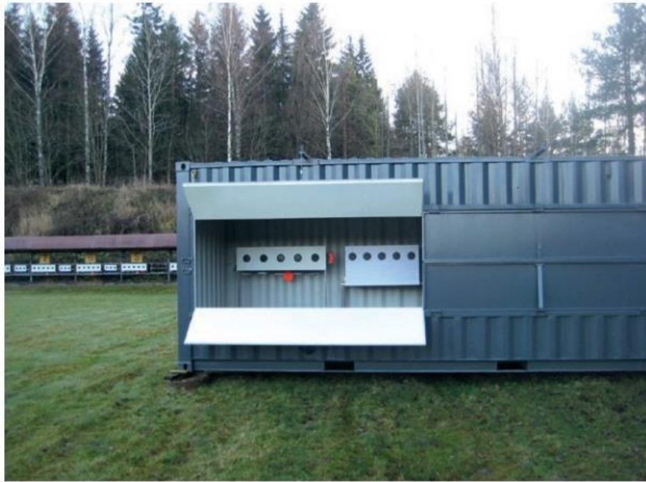
Figure A.8 Example of a prototype of biathlon target equipment and bullet traps installed in a shipping container (Kajander and Parri, 2014)
