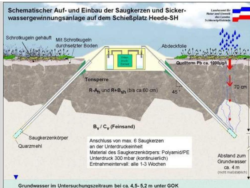
Figure A.11 Example for measurement of seepage water in a shooting range (Schleswig- Holstein LANU, 2005)
