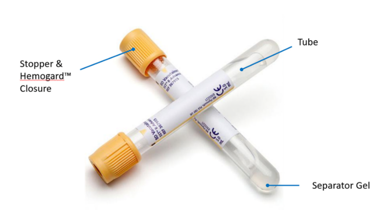
Figure 3-2 Blood collection tube components
