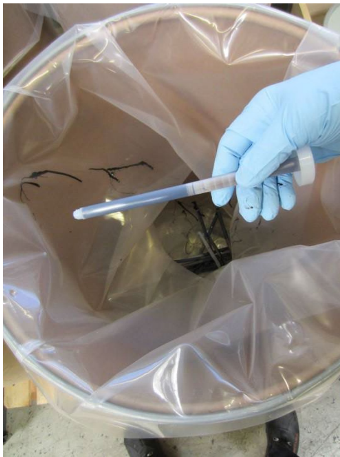
Figure 15: A worker disposing of the dasher rod and piston rod as hazardous waste
