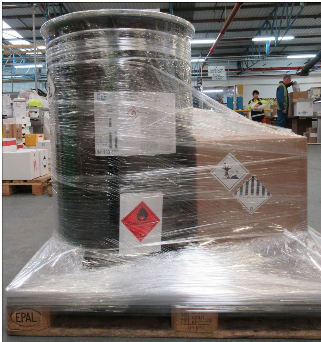
Figure 17: Example of drums used for bulk scale mixing. One large drum of base and one small drum of hardener constitute one kit.
