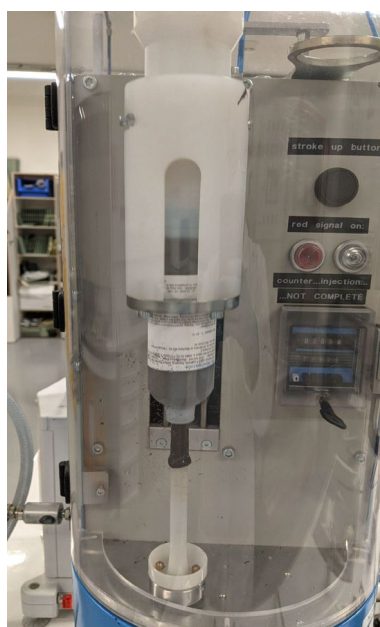
Figure 12: Machine used for mixing of two-compartment sealant kits
