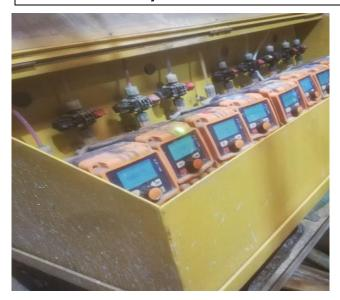
Pump system used to avoid manual handling of Chromium Trioxide containing formulations. If a problem occurs can be switched of externally to the pump container by an isolation switch for each pump to avoid being splashed, Dosing replaces manual additions where possible and should always be use for IBCs.
