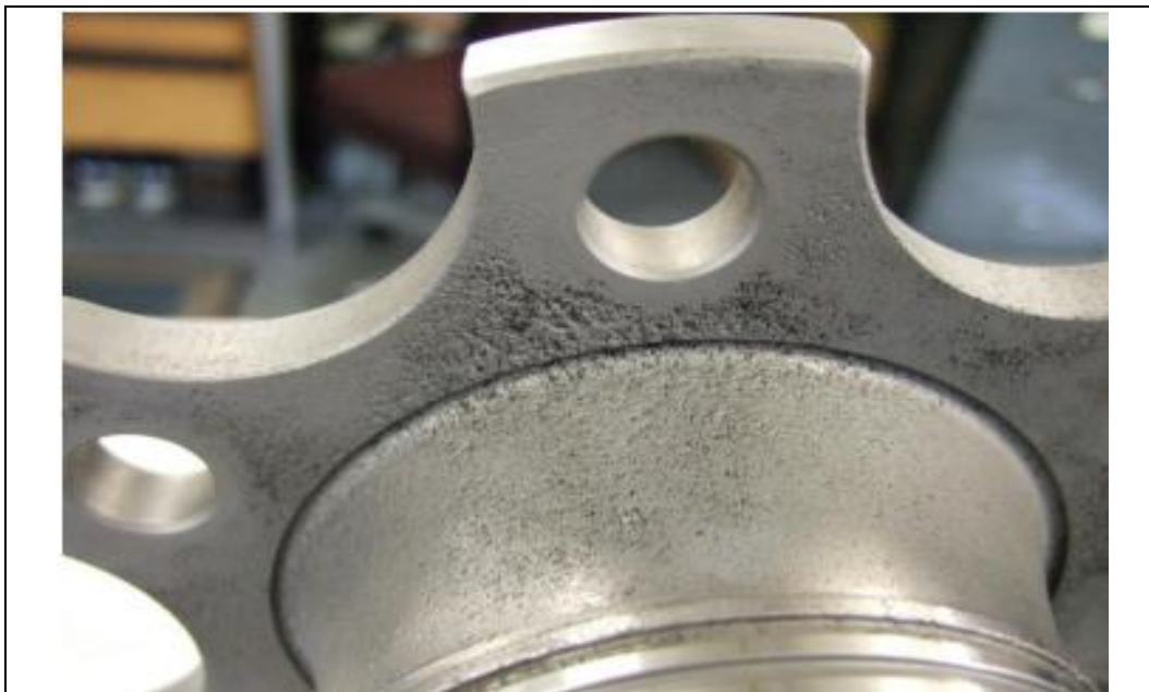
Figure 3-8: Pitting corrosion on vintage aircraft crankshaft (Civil Aviation Authority, 2017)
