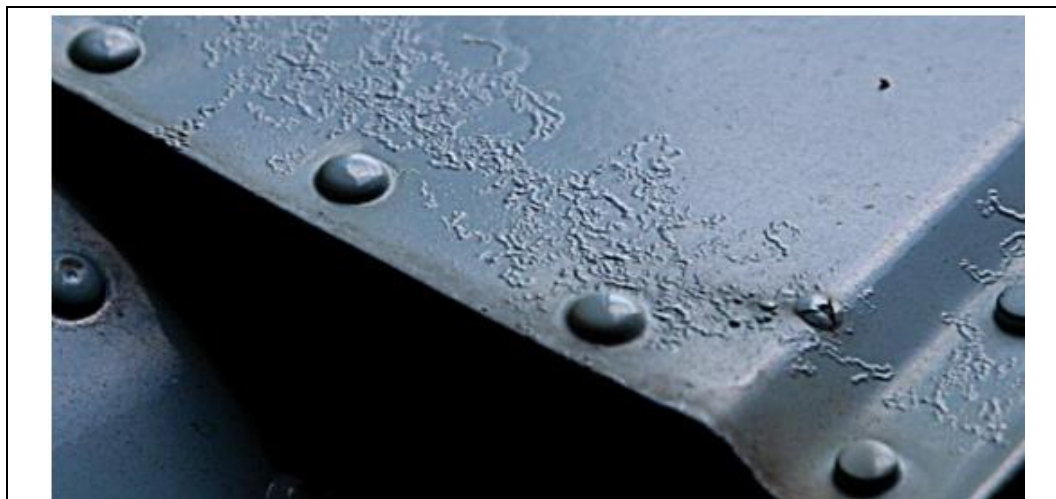
Figure 3-6: Filiform corrosion (Civil Aviation Authority, 2017)
