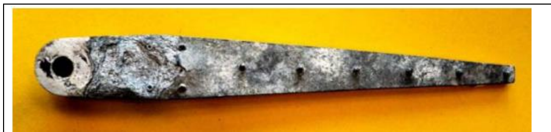
Figure 3-5: Galvanic corrosion of aluminium alloy fitting (Civil Aviation Authority, 2017)
