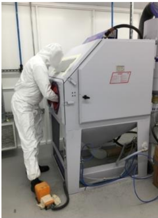
Figure 9-8: Media blasting in closed cabinet
