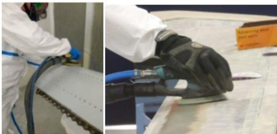
Figure 9-5: Manual abrasion performed in an extraction booth
