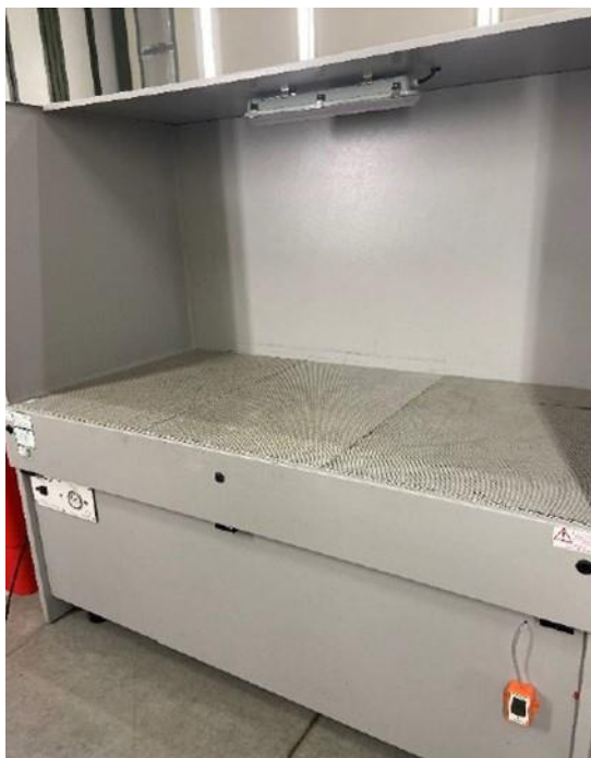
Figure VIII-8: Workbench with downdraft dust extraction
