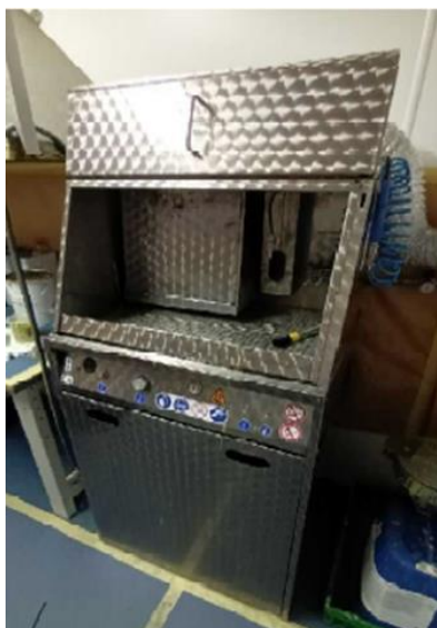
Figure VIII-5: Spray gun cleaning unit
