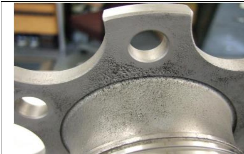
Figure 3-8: Pitting corrosion on vintage aircraft crankshaft (Civil Aviation Authority, 2017)
