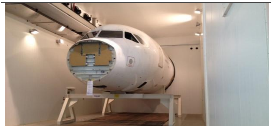
Figure 3-14: Multi-climate chamber for simulated environment testing (Airbus SAS, 2022)
