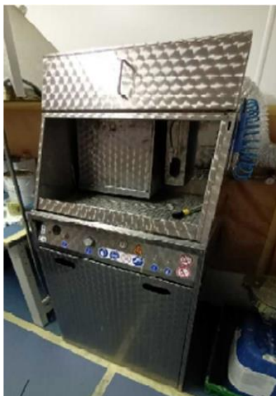
Figure VIII-5: Spray gun cleaning unit
