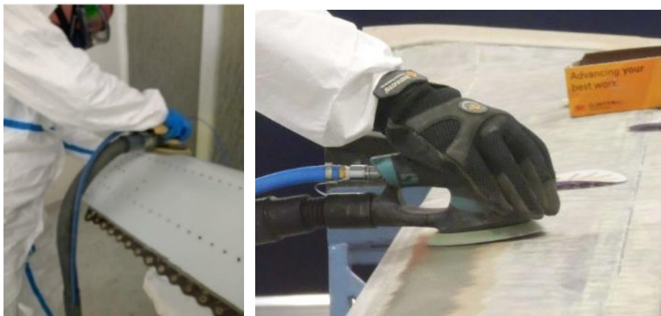
Figure 9-5: Manual abrasion performed in an extraction booth
