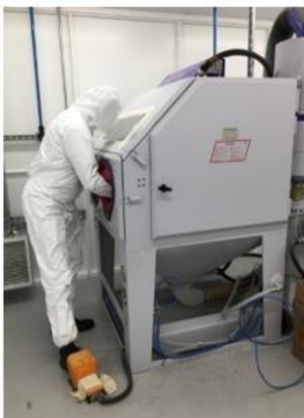
Figure 9-8: Media blasting in closed cabinet
