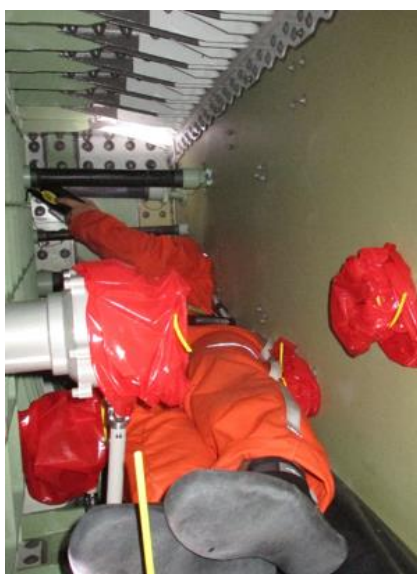
Figure 9-6: Machining performed in a confined space (wing tank)
