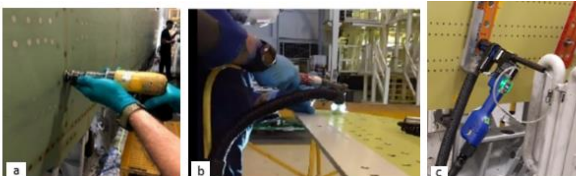
Figure 9-7: Different types of machining activities on parts (Bolting (a), deburring (b), rib drilling (c))
