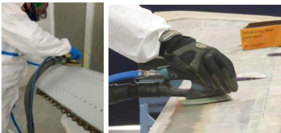
Figure 9-5: Manual abrasion performed in an extraction booth
