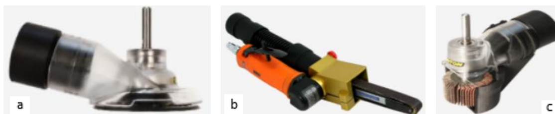
Figure 9-3: Examples of tools used for machining on surfaces (Rotary sander (a), flap wheel sander (b), band sander (c), all equipped with on-tool extraction)
