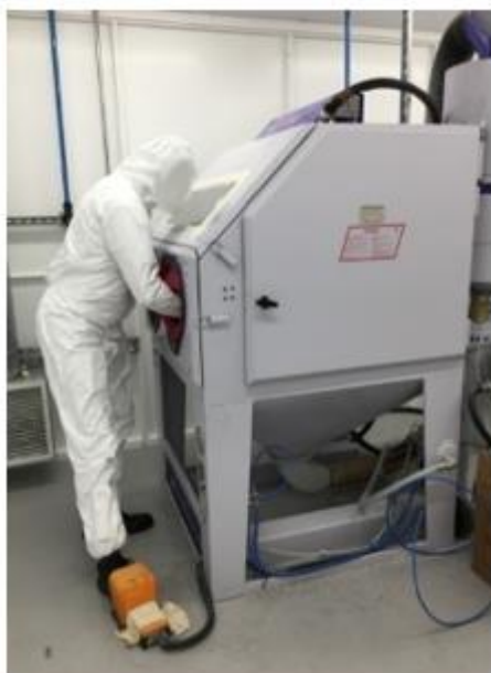
Figure 9-8: Media blasting in closed cabinet
