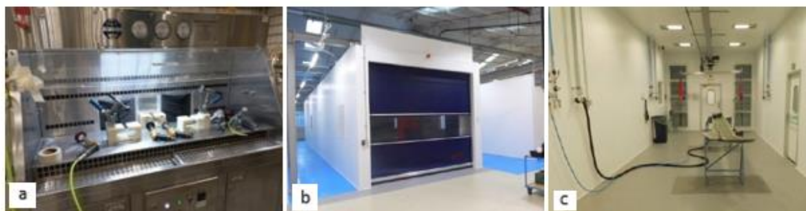
Figure 9-4: Extraction bench (a) and fettling booth (b + c) used for machining
