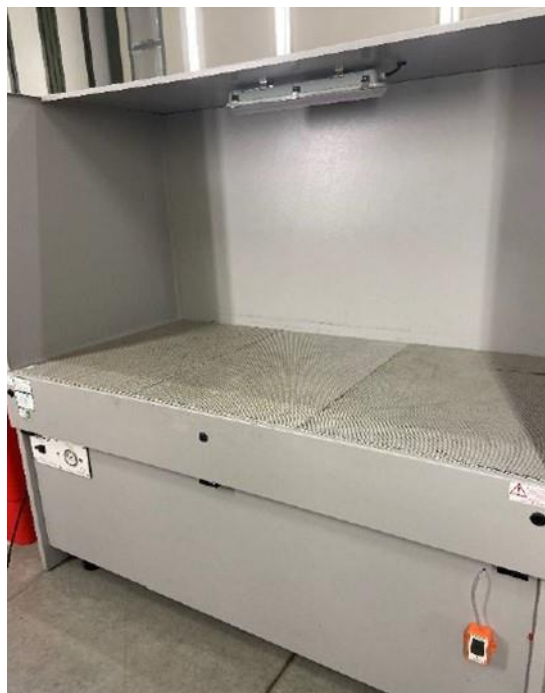
Figure VIII-8: Workbench with downdraft dust extraction
