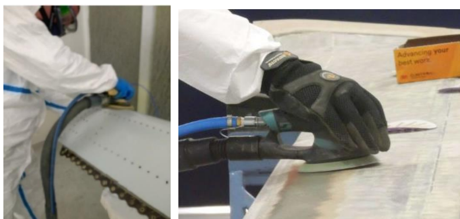
Figure 9-5: Manual abrasion performed in an extraction booth
