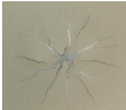
Figure 3-16: Photographic evidence of failed performance of a proprietary Cr(VI)-free test candidate in temperature resistance and mechanical properties showing unacceptable brittleness and loss in adhesion
