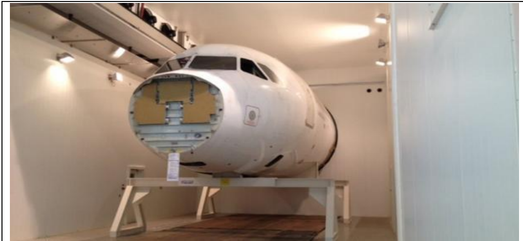
Figure 3-8: Multi-climate chamber for simulated environment testing (Airbus SAS, 2022)
