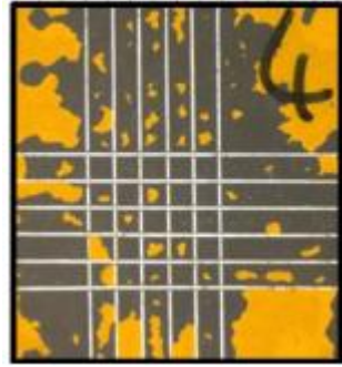
Figure 3-15: Photographic evidence of the loss in adhesion of a Cr(VI)-free wash primer from the test coupon substrate according to ISO 2409 following submersion in water
