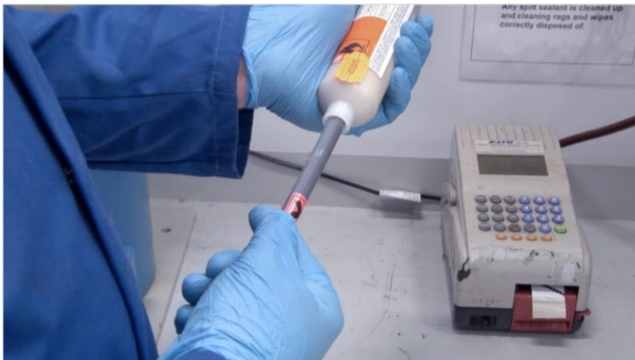
Figure 12: Insertion of the piston rod into the cartridge body by a worker
