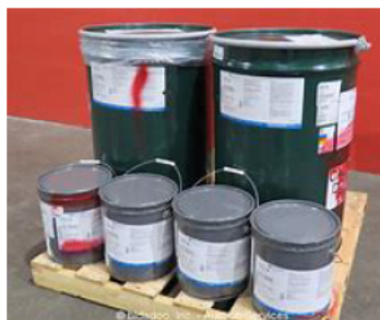
Figure 19: Example of drums used for bulk scale mixing. One large drum of base and one small drum of hardener constitute one kit
