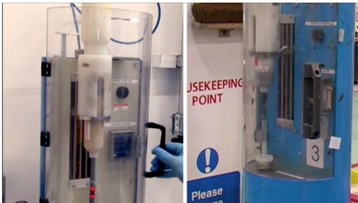
Figure 15: The mixing machine door is closed, fully containing the Techkit during mixing
