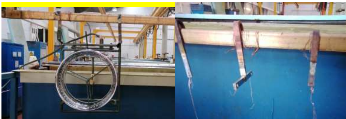
Typical Plating Jig with component
