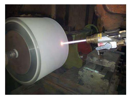
It can clearly be seen that this process is not suitable for complex geometries and internal surfaces.
