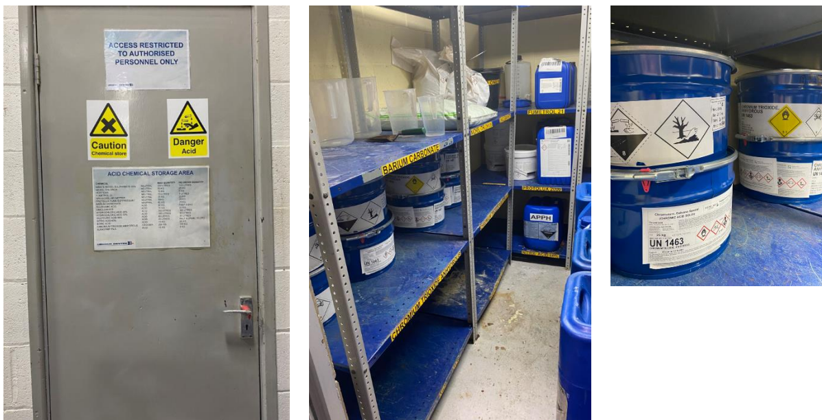
Figure 6. Photos of (a) the acid storage area, (b) the sealed CrO 3 drums on shelves in the storage room and (c) labels on the drums
