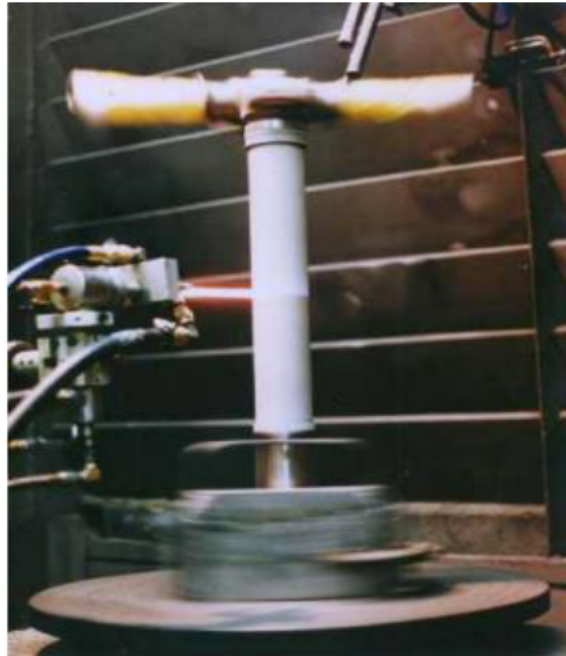
Figure 14. HVOF spray of landing gear inner cylinder 13
