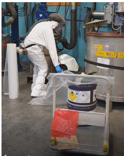
Figure 9-3: Folding the foil around the vessel after the filling process is complete
