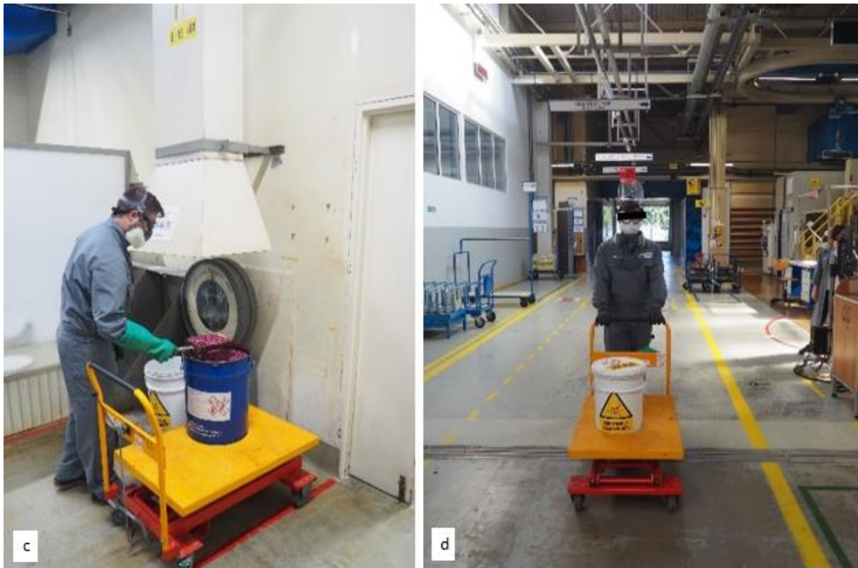
Figure 9-9: Storage room for chemicals (a), measuring and weighing of solid chromate (b + c) in a dedicated area, transport of solid chemicals to the treatment bath(s) (d)
