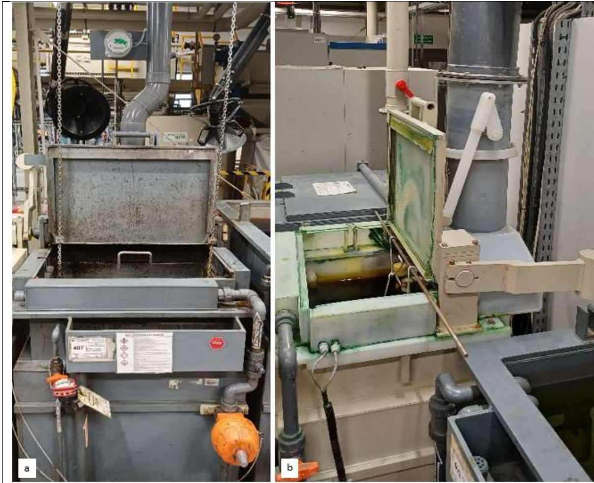
Figure 2-1: Treatment baths for inorganic finish stripping
