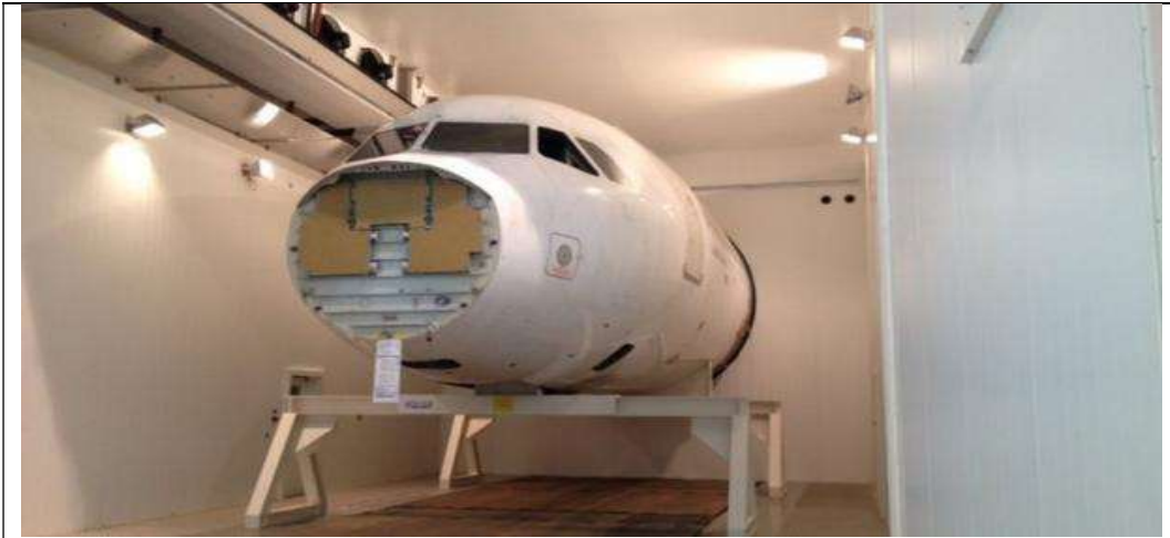
Figure 3-5: Multi-climate chamber for simulated environment testing (Airbus SAS, 2022)
