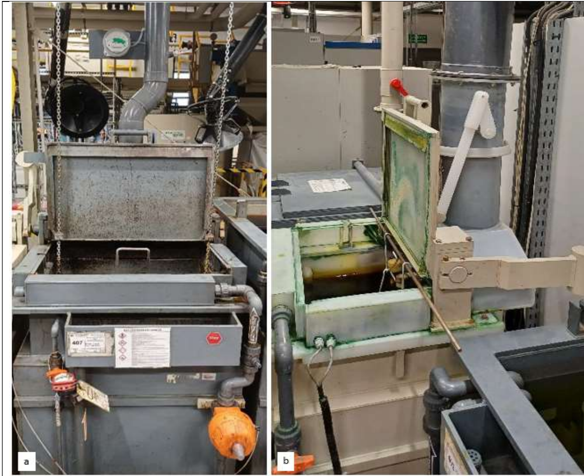
Figure 2-1: Treatment baths for inorganic finish stripping
