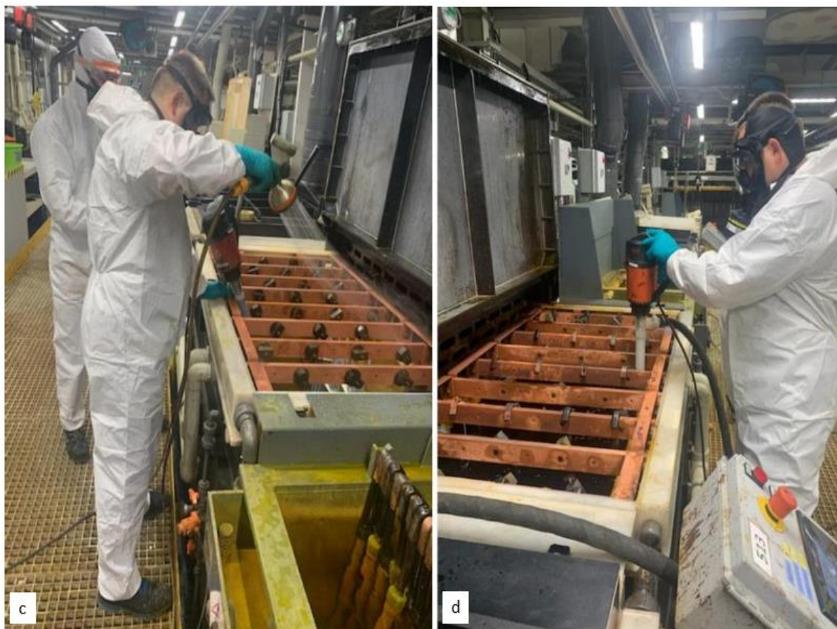
Figure 9-12: Bath emptying by transfer of old bath solution into an IBC (a) and bath cleaning with a hose and wet and dry vacuum cleaner (b, c, d)
