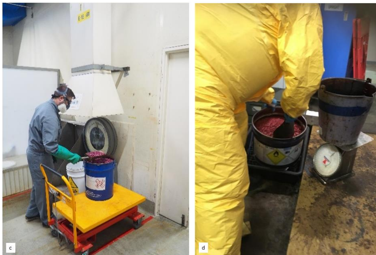
Figure 9-8: Storage room for chemicals (a), measuring of liquid chromate (b), measuring, and weighing of solid chromate (c + d) in a dedicated area
