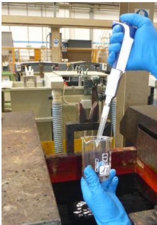
Figure 9-6: Sampling with a pipette for smaller volumes
