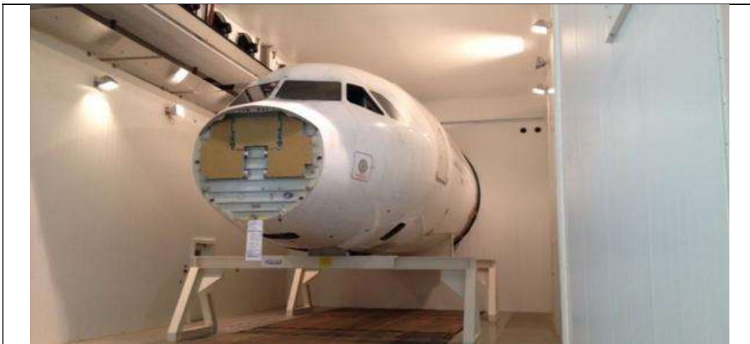
Figure 3-6: Multi-climate chamber for simulated environment testing (Airbus SAS, 2022)
