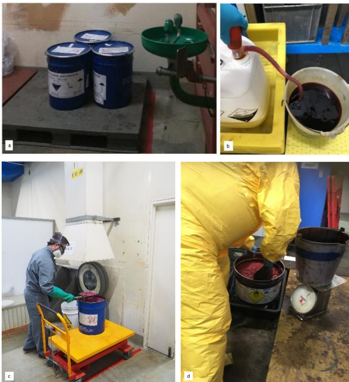
Figure 9-9: Storage room for chemicals (a), measuring of liquid chromate (b), measuring, and weighing of solid chromate (c + d) in a dedicated area
