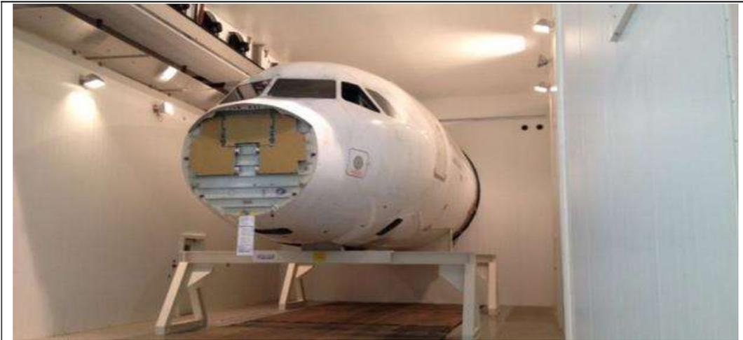
Figure 3-7: Multi-climate chamber for simulated environment testing (Airbus SAS, 2022)
