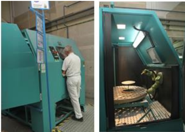
Figure 11-2: Burnishing of a slurry coated part in a closed system
