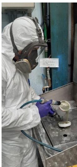
Figure 9-8: Spray operator performs manual cleaning of spray gun with water
