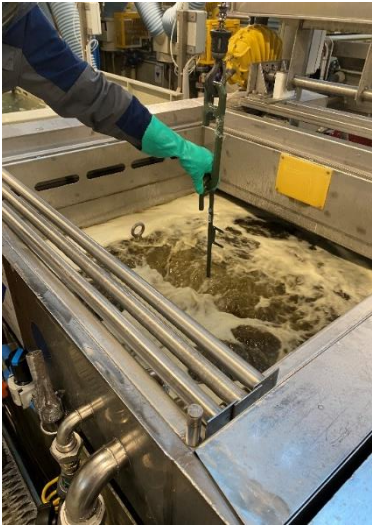
Figure 11-3: Stripping of slurry coating paint from a part by immersion in a Cr(VI)-free treatment bath
