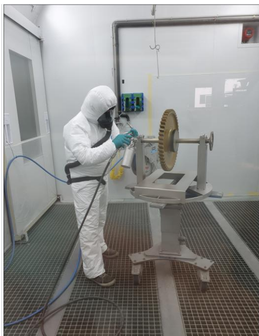
Figure 9-2: Manual spray application of slurry coating in a spray booth
