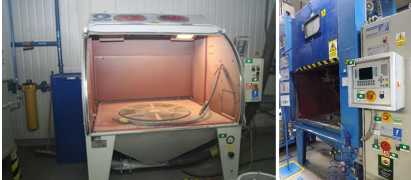
Figure 11-1: Pre-treatment by sand blasting of parts to be treated with slurry coating paint either manually (left) or automatic (right) in closed systems
