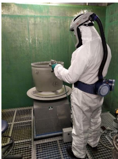
Figure 9-4: Manual spraying with slurry coating paint in a spray booth with water curtains
