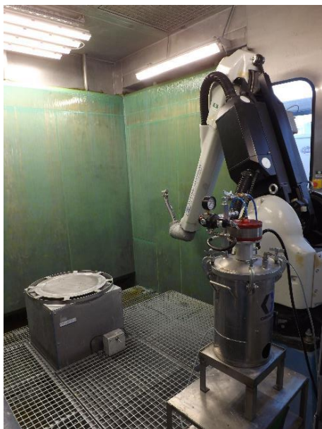
Figure 9-5: Robot for automated spraying of slurry coating paint in a closed spray booth with running water curtains
