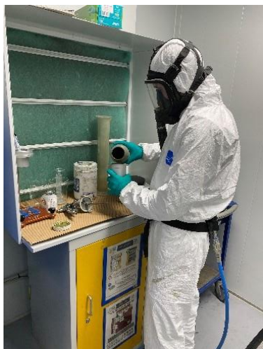
Figure 9-7: Filling of spray gun reservoir by decanting slurry coating paint at a workbench connected to LEV
