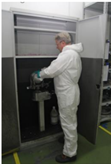
Figure 9-6: Spray operator fixing a closed slurry coating paint container in a shaker
