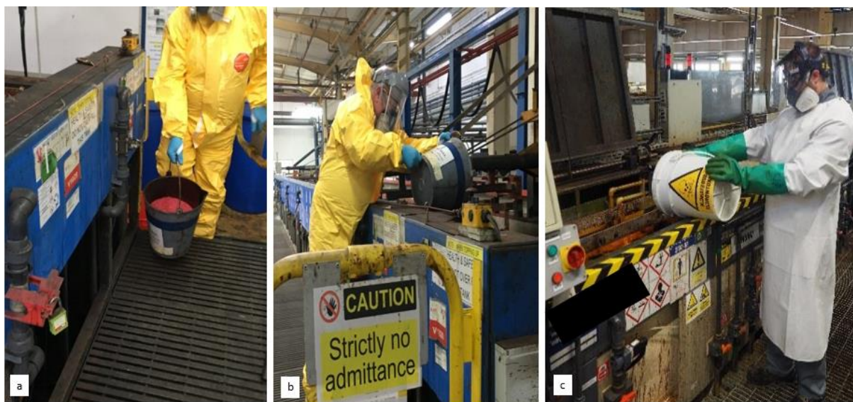
Figure 9-11: Operator transfers a bucket with solid chromate to the tank (a); operator carefully pours the chromate into the bath for bath make-up or addition (b + c)
