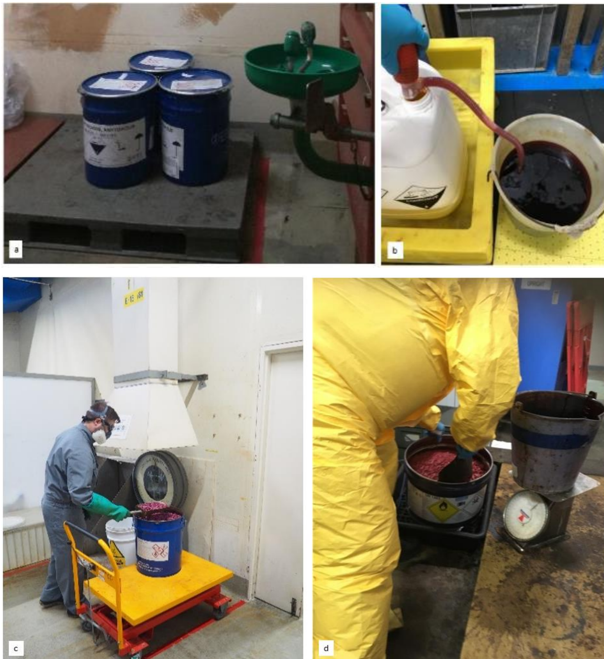
Figure 9-8: Storage room for chemicals (a), measuring of liquid chromate (b), measuring, and weighing of solid chromate (c + d) in a dedicated area
