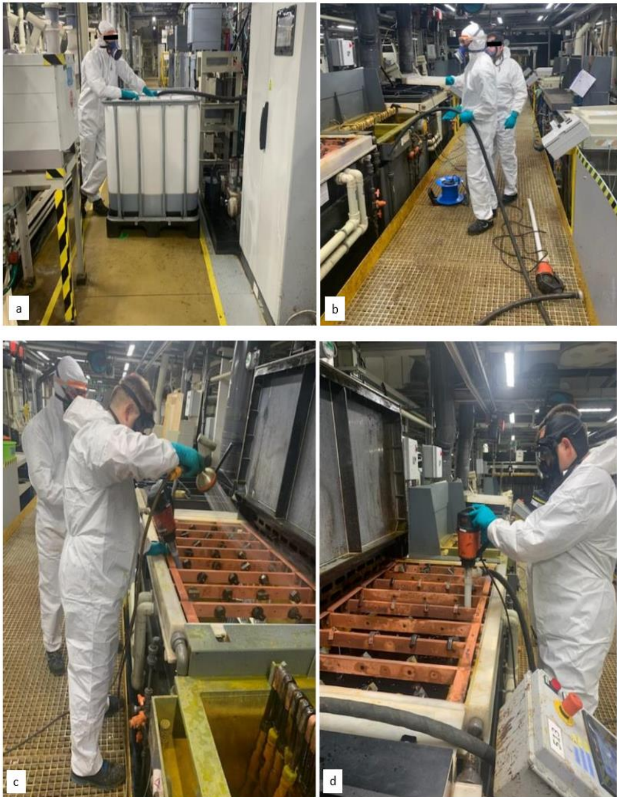
Figure 9-12: Bath emptying by transfer of old bath solution into an IBC (a) and bath cleaning with a hose and wet and dry vacuum cleaner (b, c, d)
