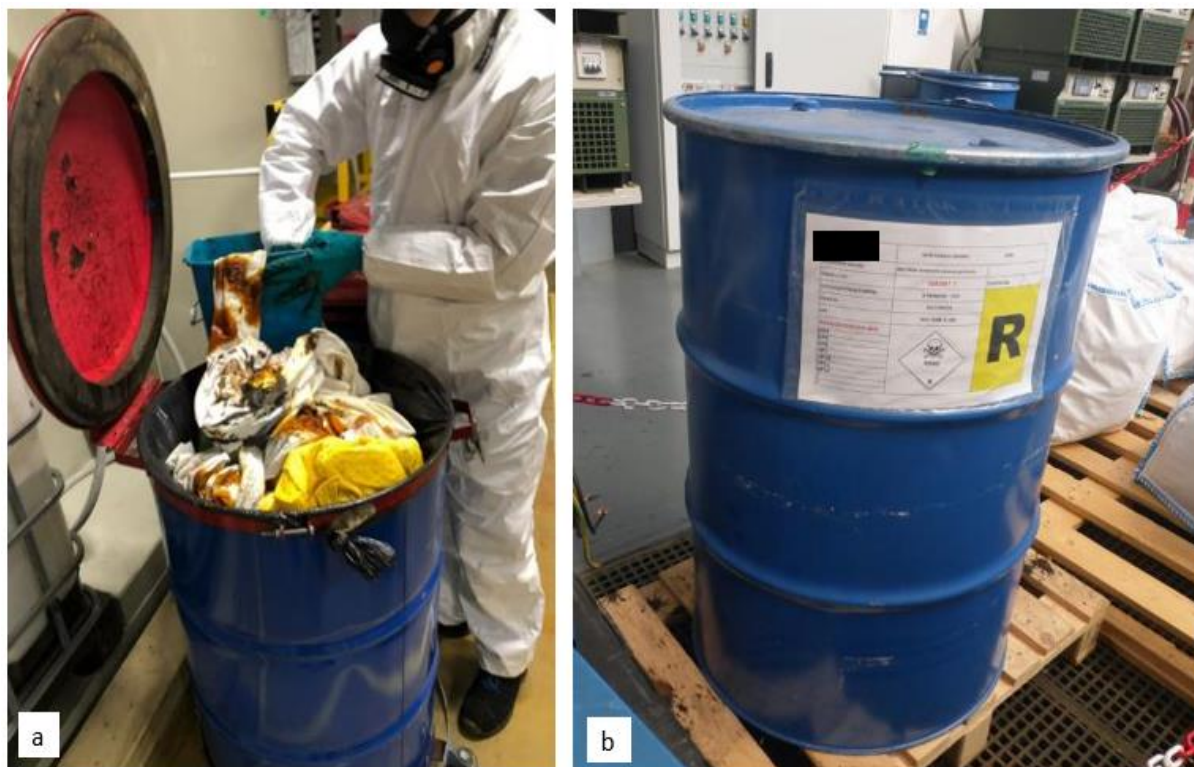
Figure 9-10: Operator discarding solid waste contaminated with Cr(VI) into a drum for hazardous waste (a); closed hazardous waste drum (b)
