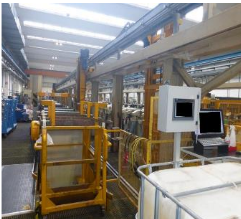
Figure 9-5: Automatic line with control area in front of automatic line (at the monitor)
