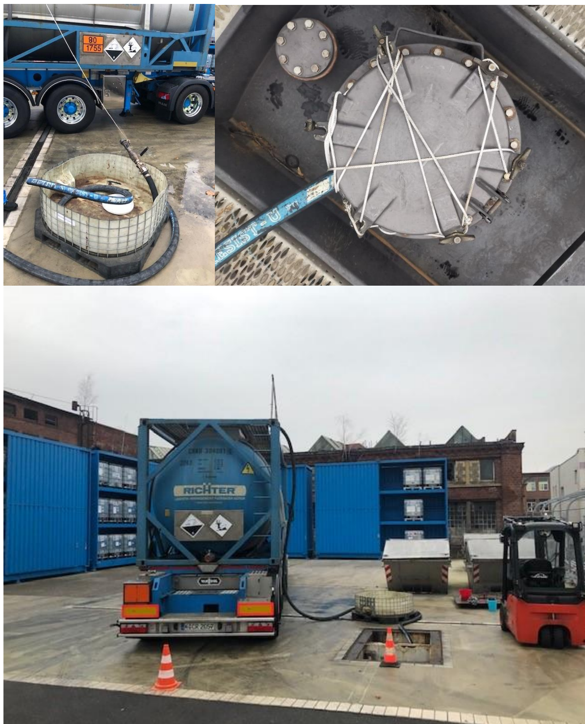
Figure 2: Loading of a tank truck
