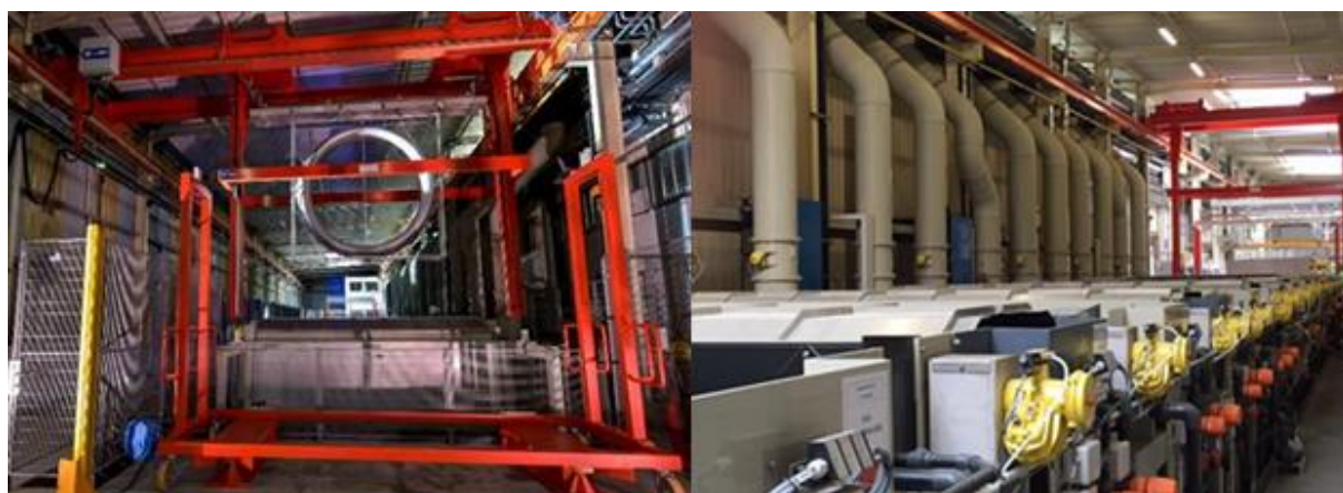
Figure 9-6: Automatic line with an immersion process controlled by a crane (a) moving along the different baths (b)
