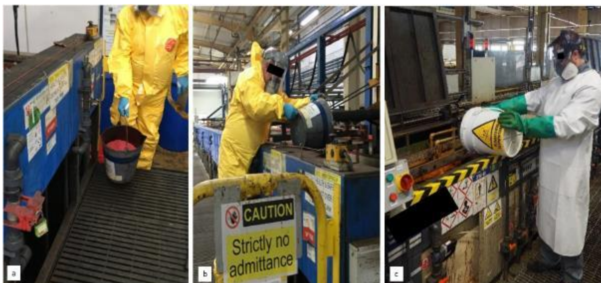
Figure 9-12: Operator transfers a bucket with solid chromate to the tank (a); operator carefully pours the chromate into the bath for bath make-up or addition (b + c)
