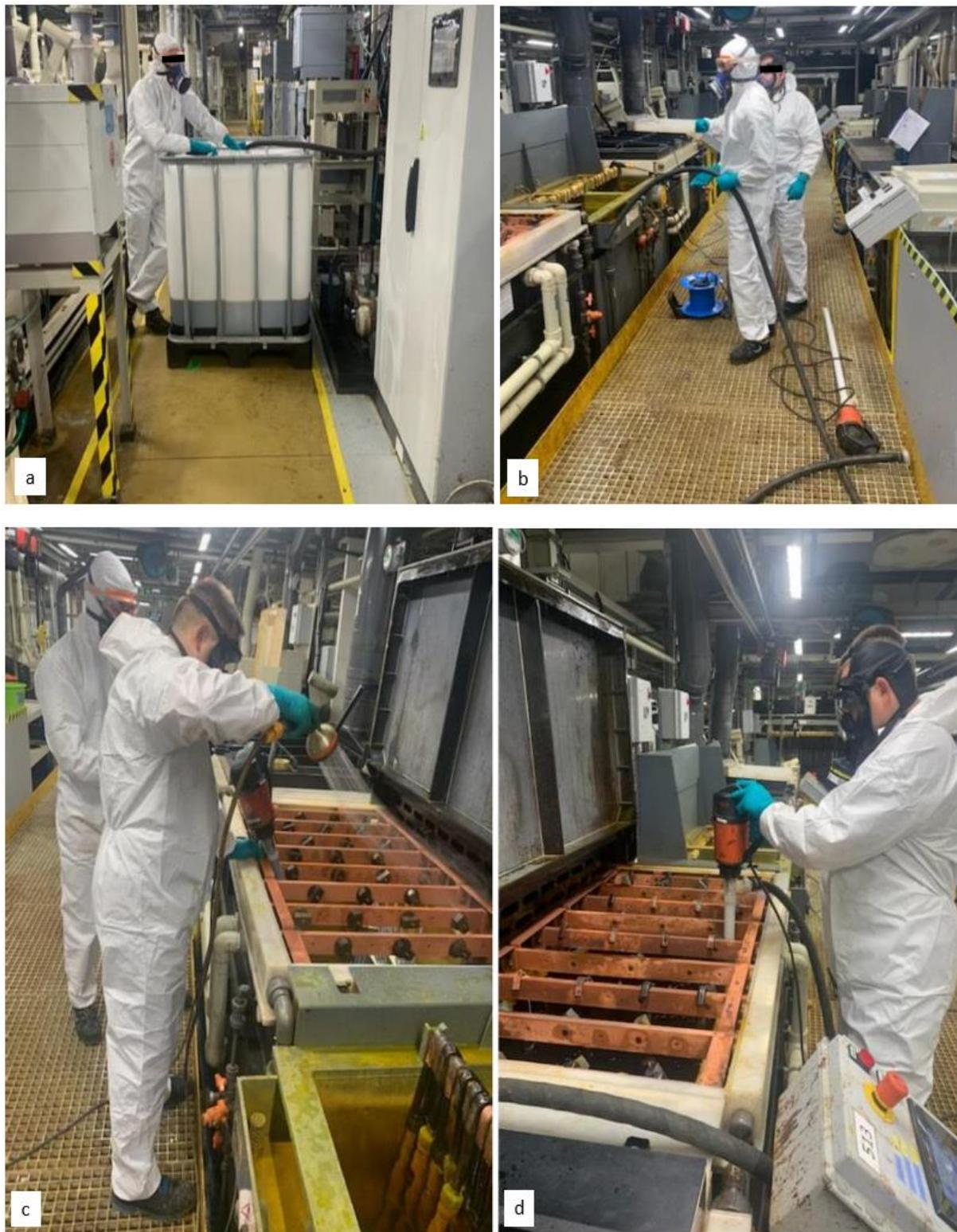
**Figure 9-10: Bath emptying by transfer of old bath solution into an IBC (a) and bath cleaning with a hose and wet and dry vacuum cleaner (b, c, d)**
