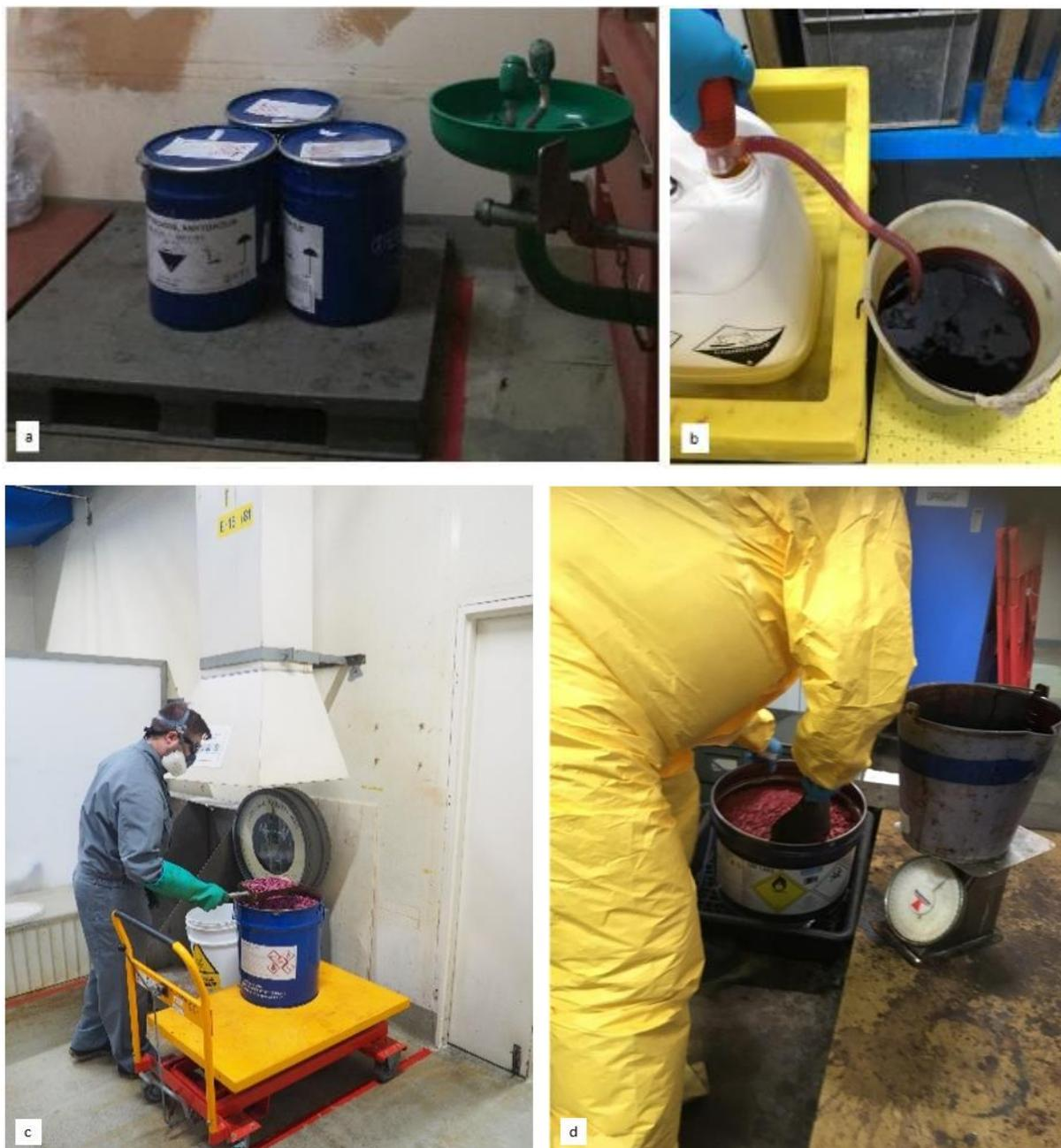
**Figure 9-6:** Storage room for chemicals (a), measuring of liquid chromate (b), measuring and weighing of solid chromate (c + d) in a dedicated area
