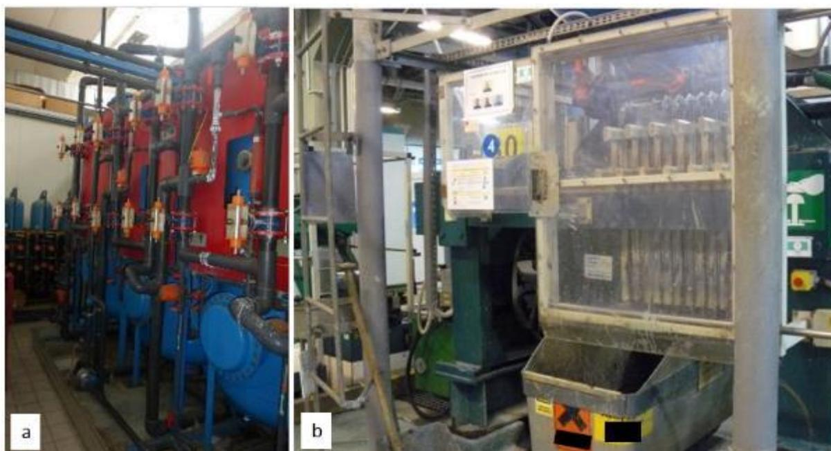
**Figure 9-3:** Water deionisation tanks for wastewater treatment (a) and filter press for separation of the filter cake (b)
