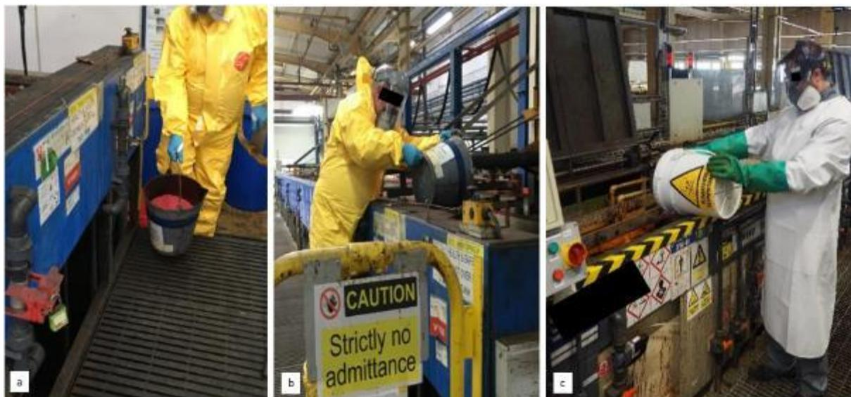
**Figure 9-9:** Operator transfers a bucket with solid chromate to the tank (a); operator carefully pours the chromate into the bath for bath make-up or addition (b + c)
