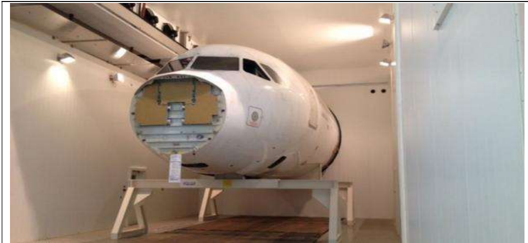
Figure 3-6: Multi-climate chamber for simulated environment testing (Airbus SAS, 2022)
