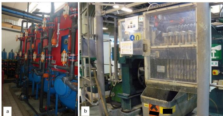
Figure 9-4: Water deionisation tanks for wastewater treatment (a) and filter press for separation of the filter cake (b)
