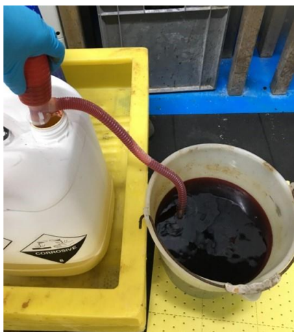
Figure 9-9: Aliquoting liquid CT with a hand pump
