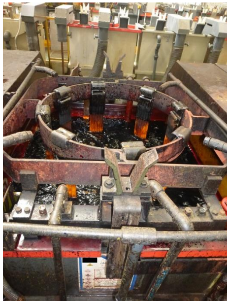
Figure 9-2: Treatment bath for electroplating with anode
