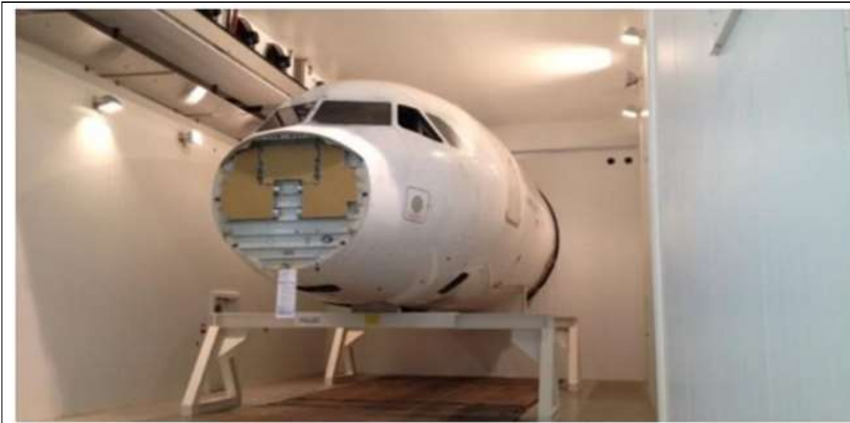
Figure 3-5: Multi-climate chamber for simulated environment testing Source: Airbus SAS 2022
