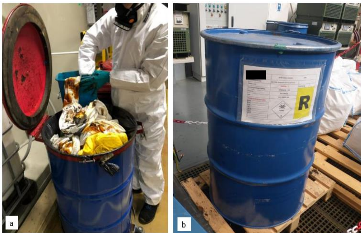
Figure 9-12: Operator discarding solid waste contaminated with Cr(VI) into a drum for hazardous waste (a); closed hazardous waste drum (b)
