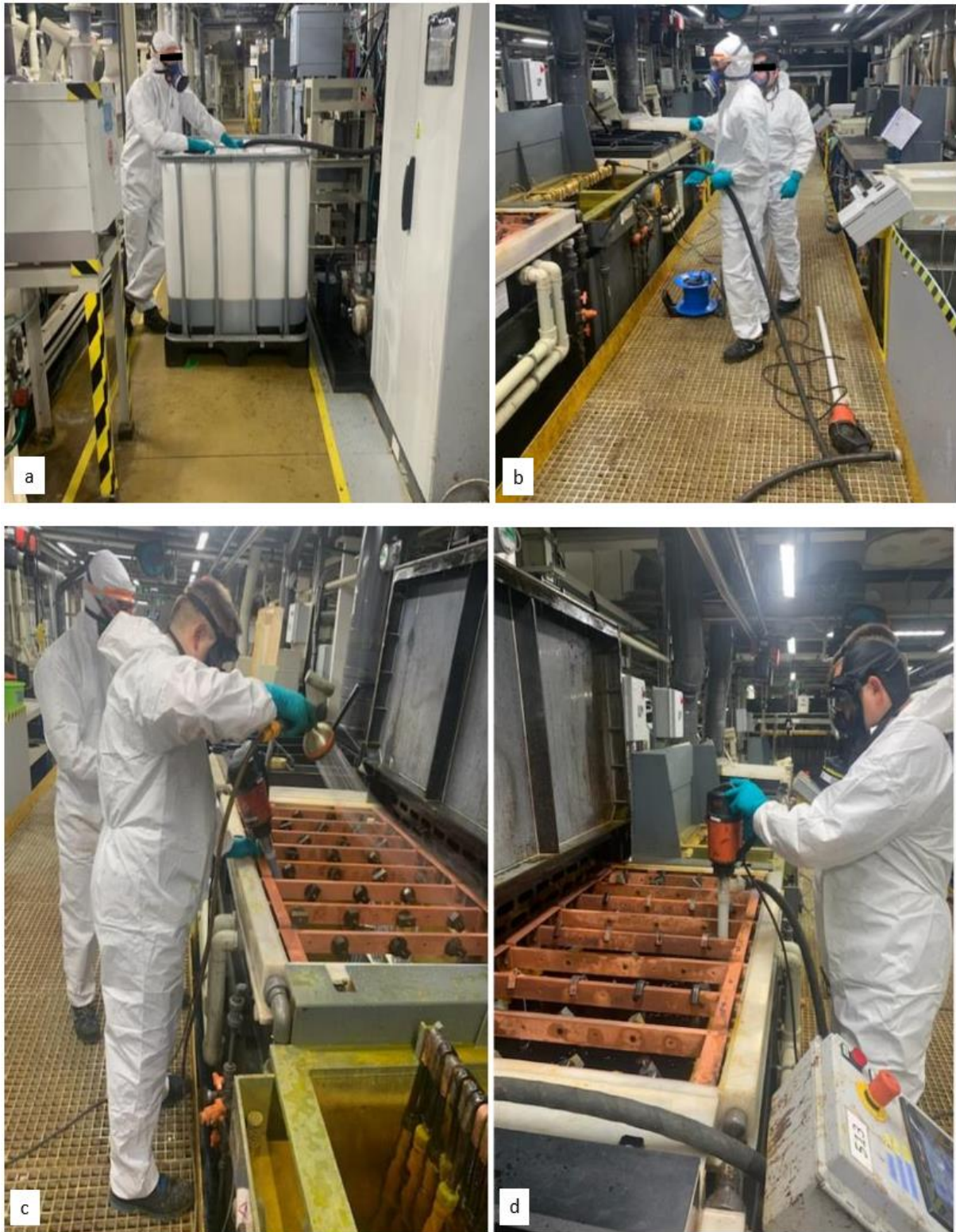
Figure 9-14: Bath emptying by transfer of old bath solution into an IBC (a) and bath cleaning with a hose and wet and dry vacuum cleaner (b, c, d)
