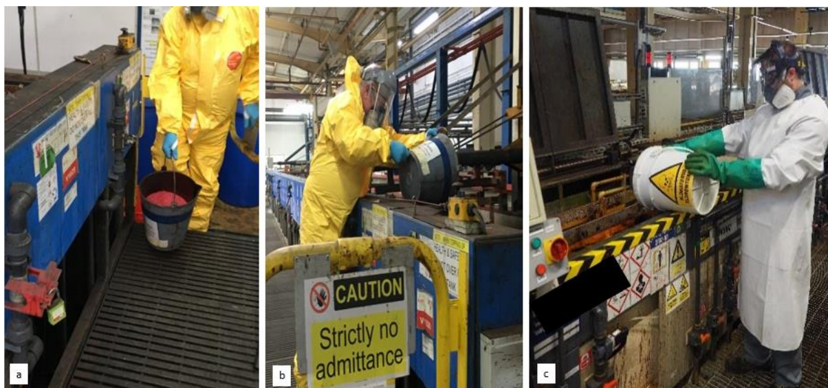
Figure 9-13: Operator transfers a bucket with solid chromate to the tank (a); operator carefully pours the chromate into the bath for bath make-up or addition (b + c)
