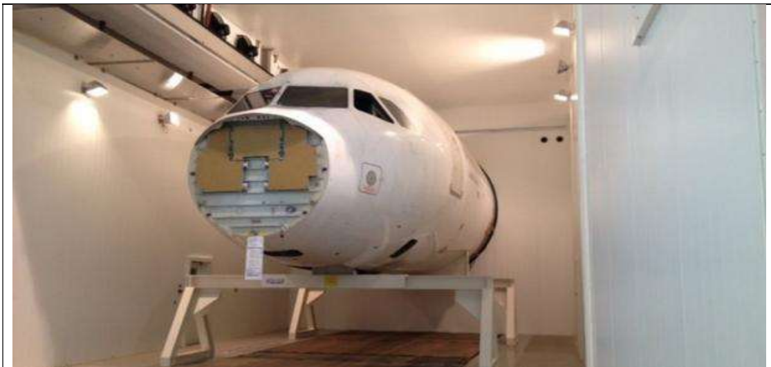
Figure 3-7: Multi-climate chamber for simulated environment testing (Airbus SAS, 2022)
