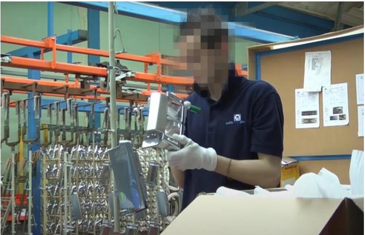
**Figure 16:** Unloading ('un-jigging') and inspection following electroplating (source: QPP)
