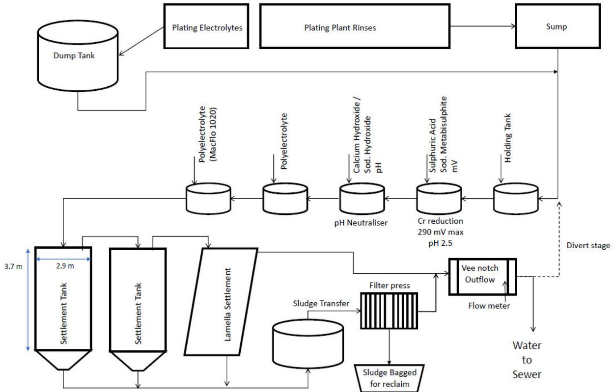
**Figure 20:** Schematic of wastewater treatment plant (source: QPP)
