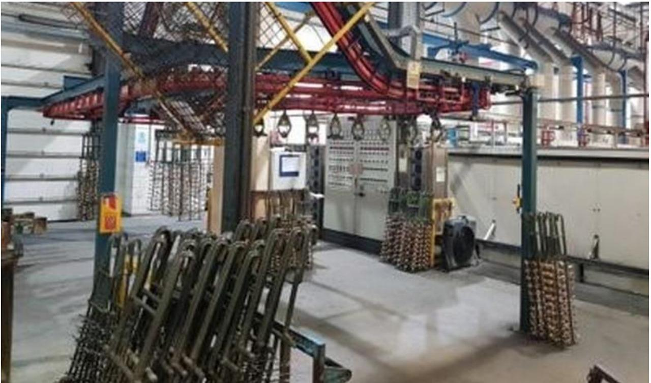
**Figure 15:** Loading ('jigging') area preceding chrome plating stage (source: Aalberts)
