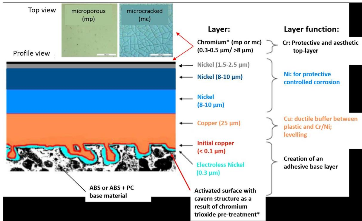
**Figure 19:** Surface of plastic substrates on completion of chrome plating (source: QPP)
