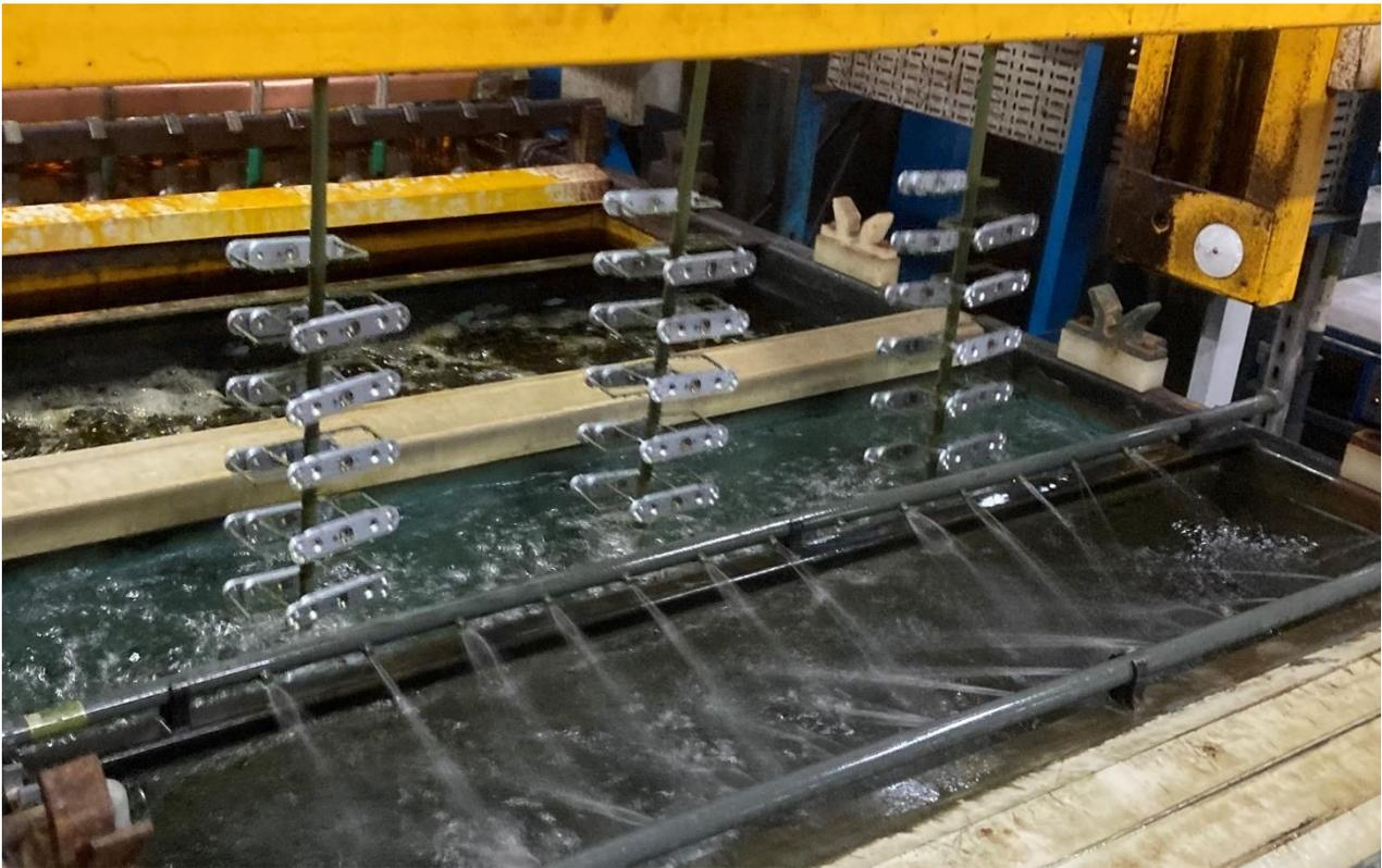
**Figure 13:** Electroplating line, detail (source: Samuel Heath)
