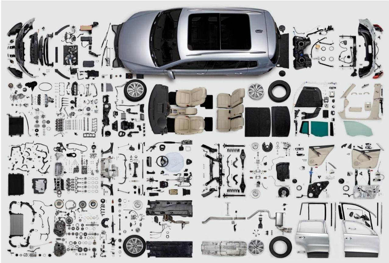
**Figure 23:** VW Tiguan disassembled into constituent parts (source: Volkswagen)
