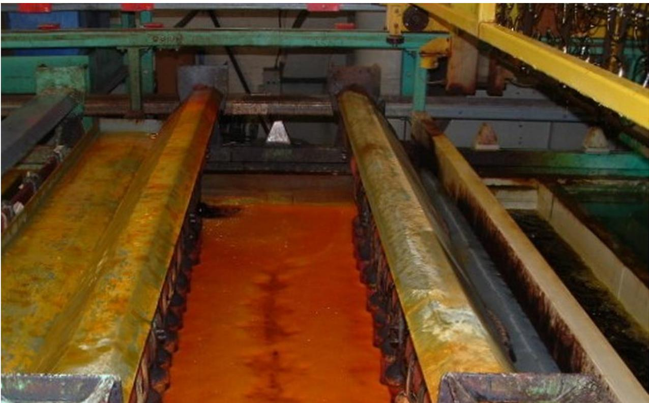
**Figure 14:** Example of a chromium bath with LEV (lip extraction) to the side and foam film which helps inhibit the release of aerosols (source: Borough)
