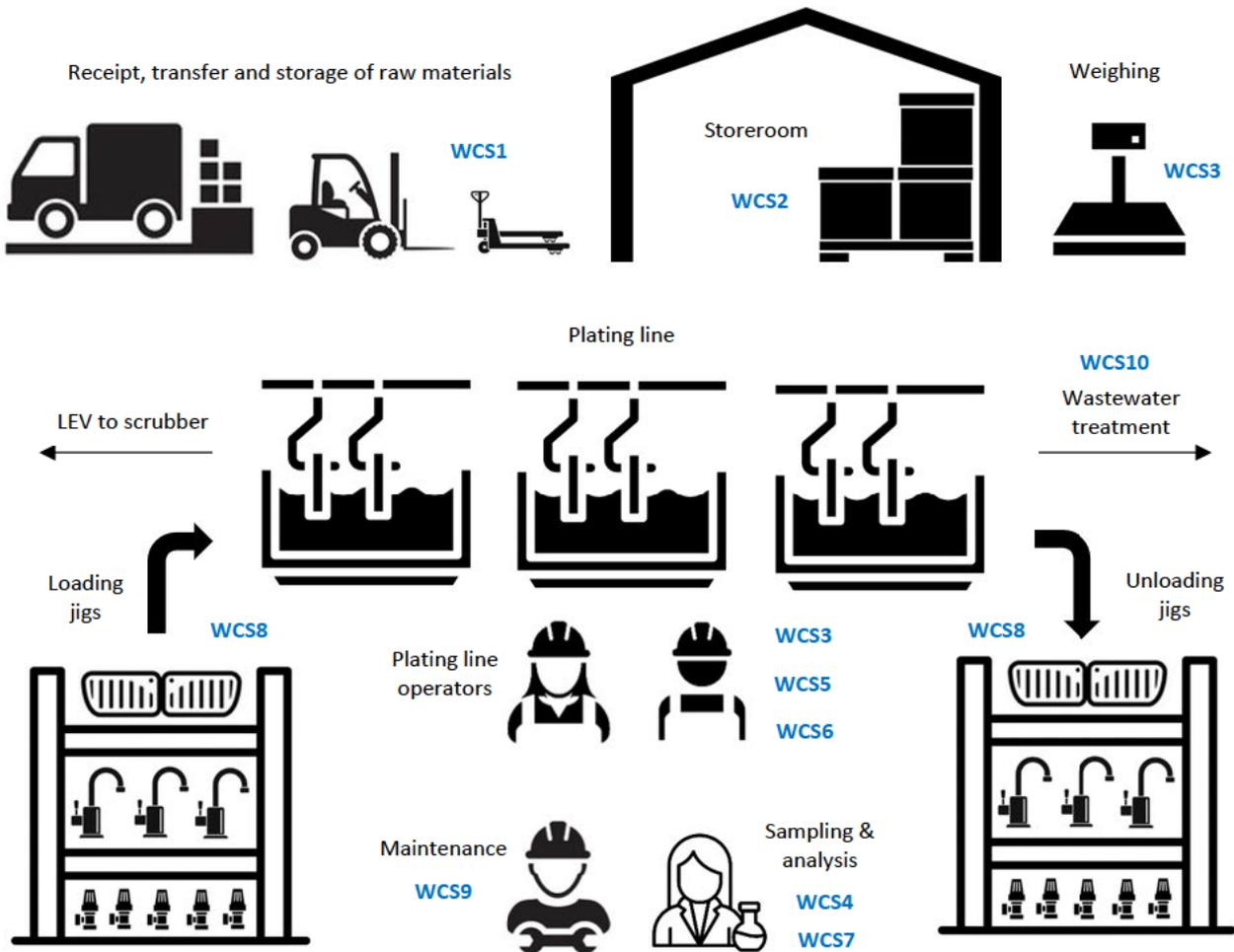
Figure 10: Schematic of the electroplating process, with references to the relevant WCS
