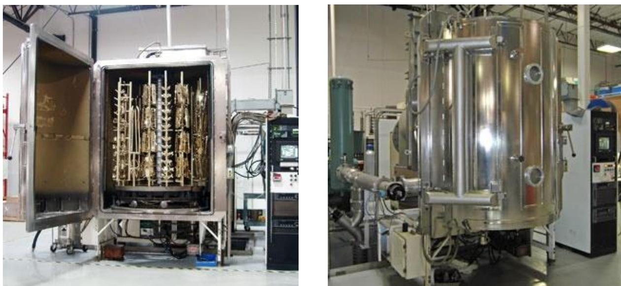
**Figure 25:** Example of a decorative batch PVD coater utilising the LTAVD process (source: [westcoastpvd.com](http://westcoastpvd.com))
