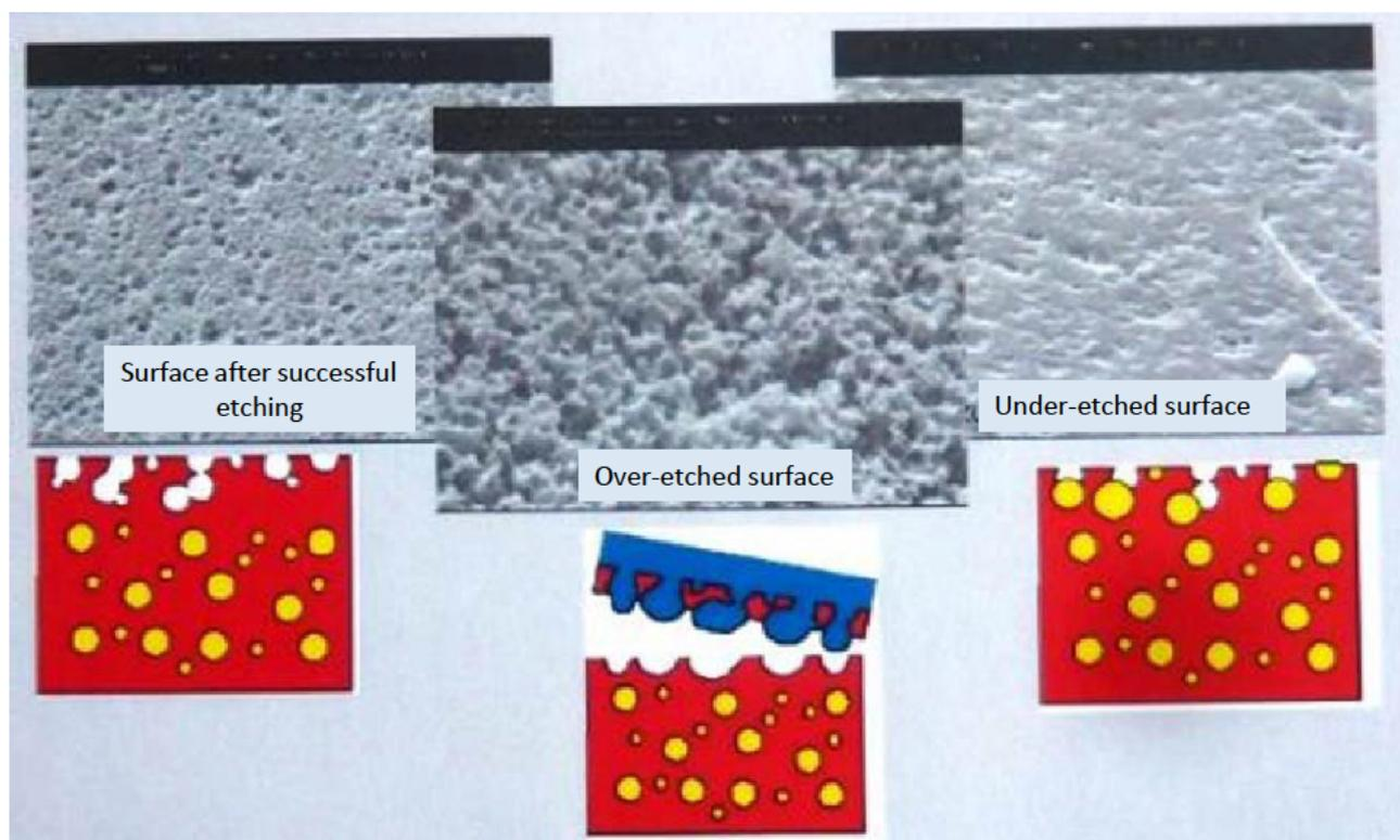
**Figure 17:** Inadequately-etched surfaces compared with a successfully-etched surface (source: QPP)
