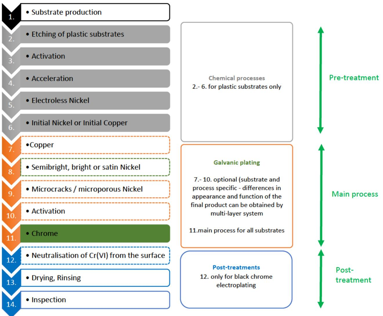
Figure 9: Process flow chart for the plating process. Data source: CTACSub
