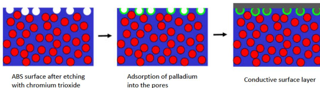
**Figure 18:** Illustration of the etching process on ABS (source: QPP)
