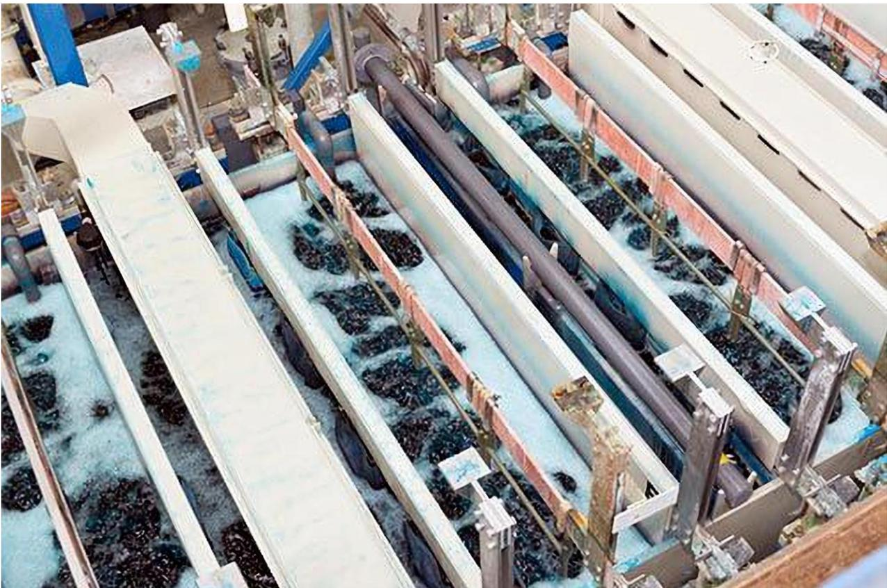
**Figure 12:** Electroplating line, detail (source: QPP)
