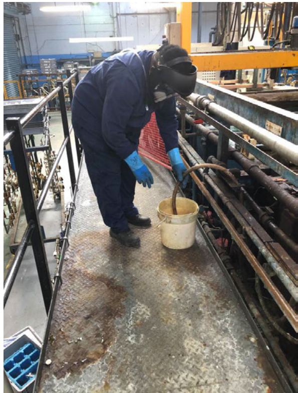
Figure 17: Container used for weighing and long lance used to ensure dissolution (L) and technician rinsing out of weighing container (R)
