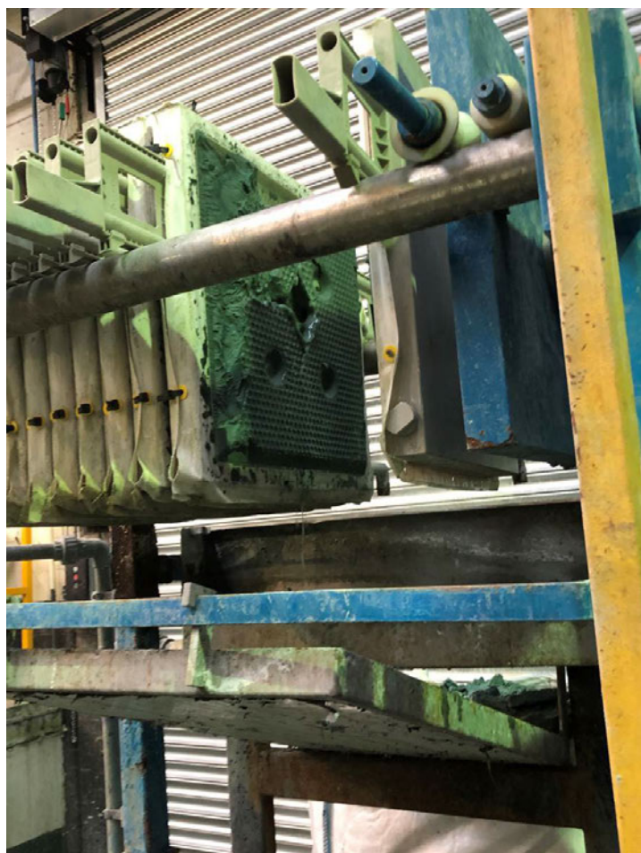
Figure 26: Photograph of sludge on filter press
