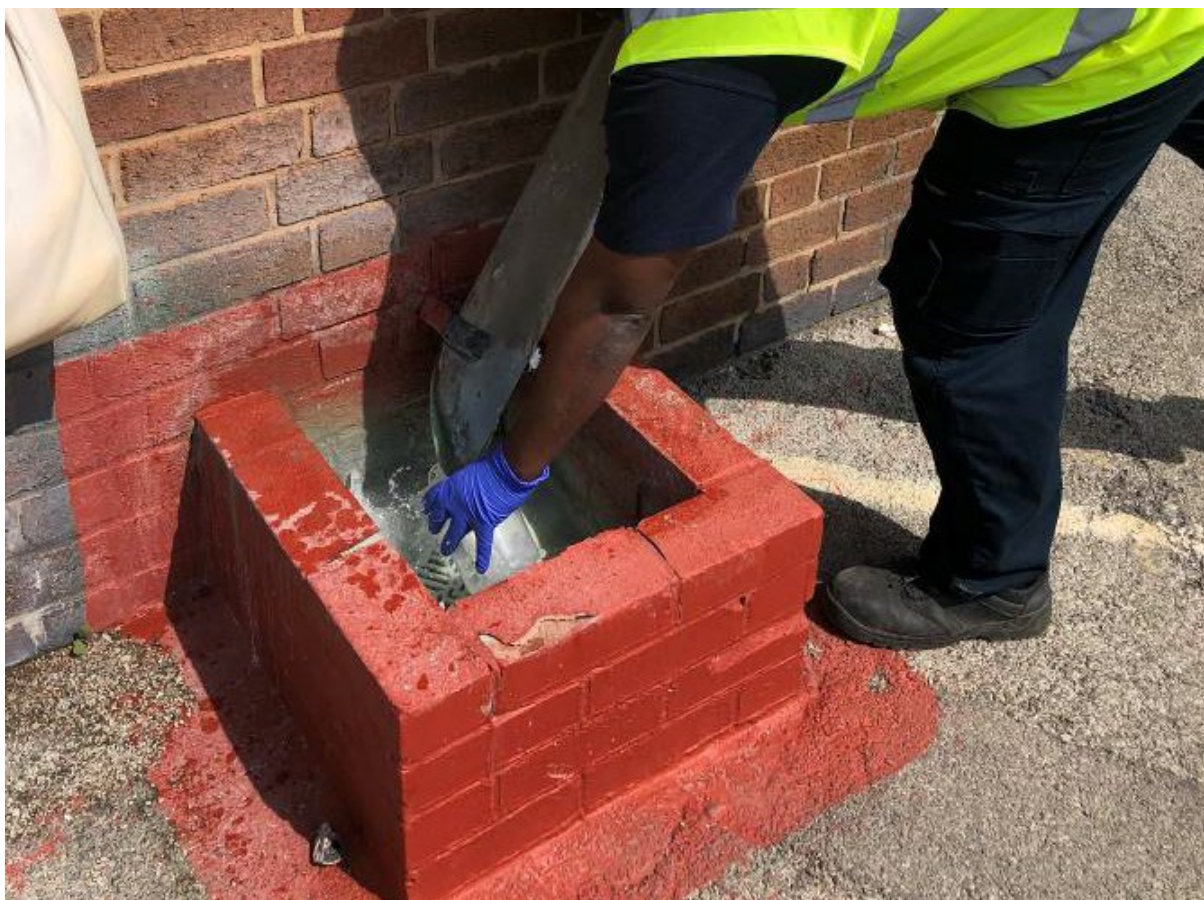
Figure 25: Photograph of a technician collecting a water sample from the final discharge point
