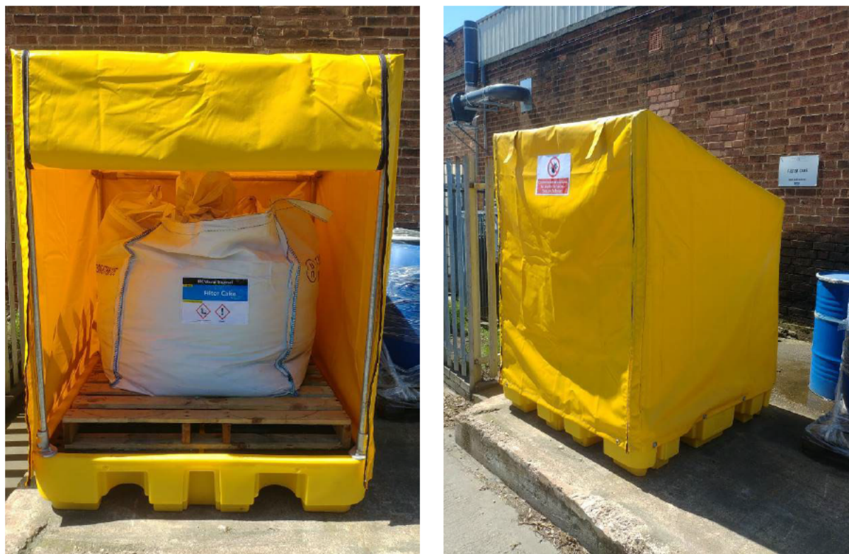
Figure 27: Photograph of sealed bag containing filter cake – signs are visible to show access is restricted
