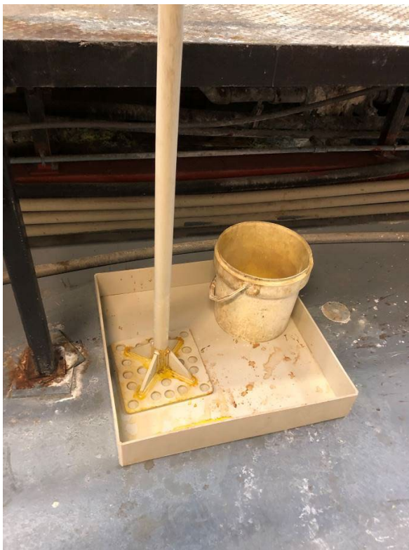
Figure 17: Container used for weighing and long lance used to ensure dissolution (L) and technician rinsing out of weighing container (R)
