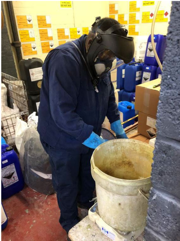
Figure 16: Weighing of chromium trioxide in chemical stores (L) and addition of the chromium trioxide flakes into the chromium plating tank (R)
