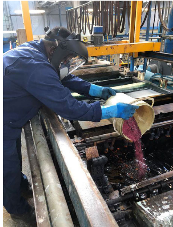
Figure 16: Weighing of chromium trioxide in chemical stores (L) and addition of the chromium trioxide flakes into the chromium plating tank (R)
