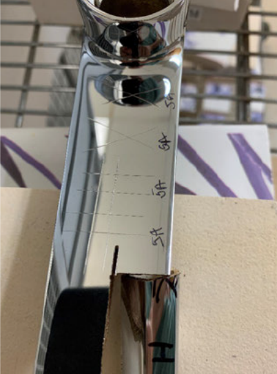
Figure 14: Results of adhesion tests on Fortune Brands parts made with hexavalent and trivalent chromium processes
