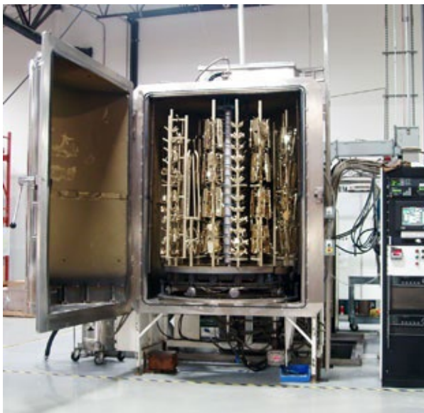
Figure 25: Example of a decorative batch PVD coater utilising the LTAVD process (source: westcoastpvd.com)
