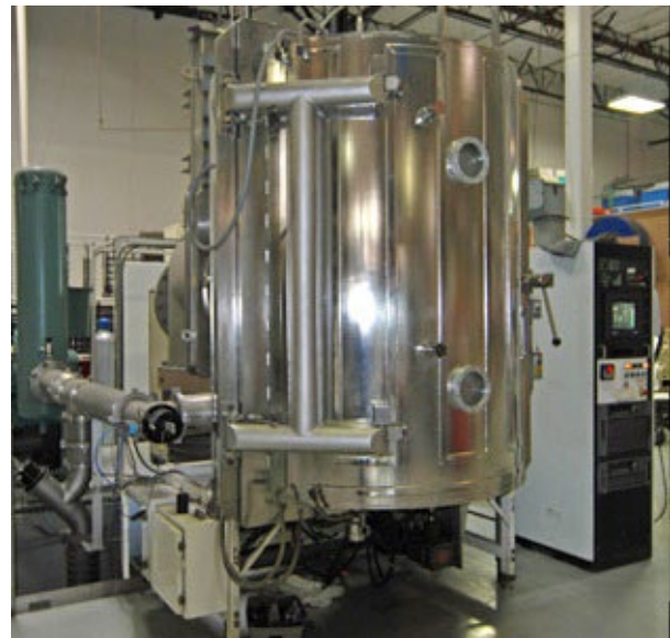
Figure 25: Example of a decorative batch PVD coater utilising the LTAVD process (source: westcoastpvd.com)
