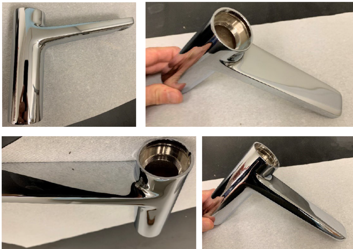
Figure 8: Results of corrosion test on Fortune Brands products made with Cr(VI) - No staining or corrosion spots observed in any of the salt spray tests
