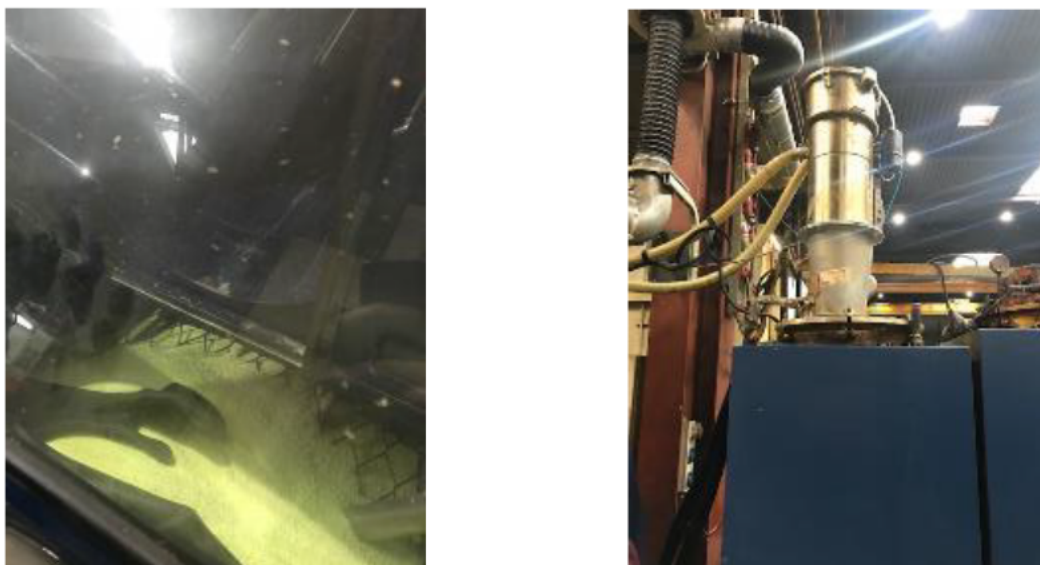
Figure 6. Photos showing (a) an operator positioning MOCA drum on MOCA feeder, the closed door at the rear of the glovebox, (c) using the gloves to open the inlay bag and (d) and MOCA storage unit in the casting machine
