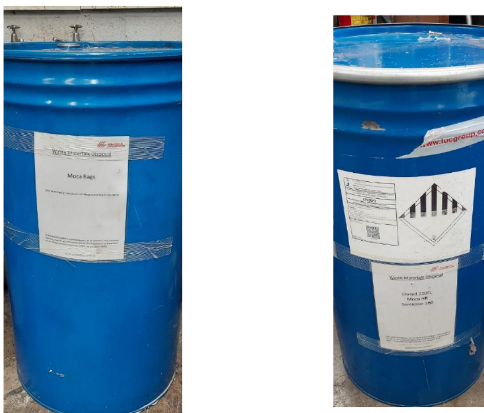
Figure 7. Photos of waste collection for MOCA inlay bags and MOCA containing waste streams
