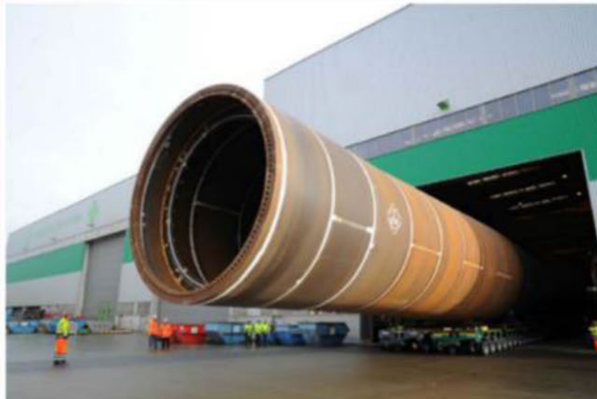
Figure 12. Monopile being transported out of manufacturing facility
