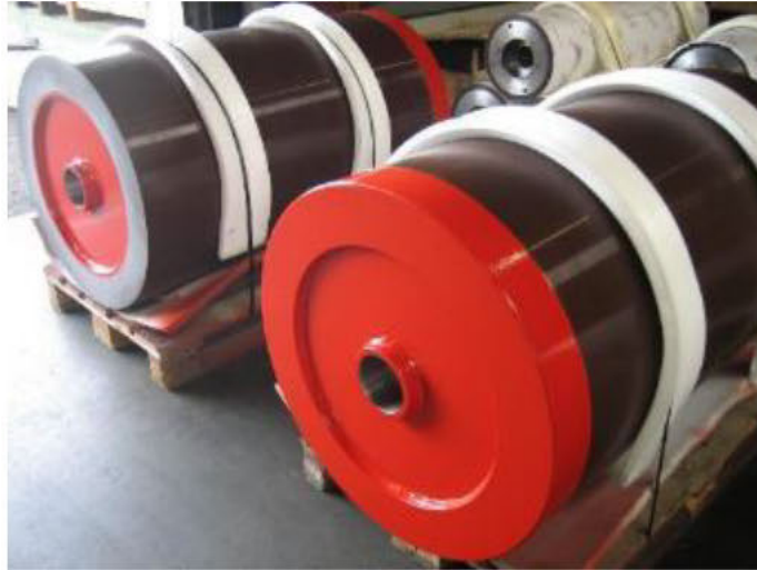
Figure 2. Example of heavy duty rollers ready for shipping. The dark coloured layer is the polyurethane. The steel roller body is in red
