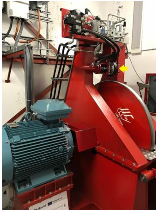
Figure 21. LUC Group's Ride Simulator. The test PU wheel is shown by an arrow
