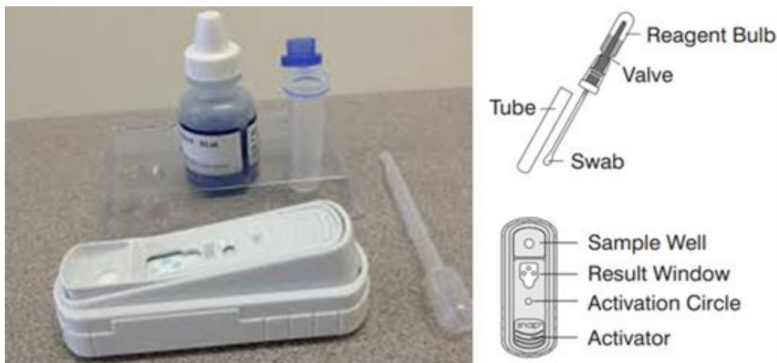
Figure 1. (left) The components of SNAP test kit for whole blood, serum, plasma and milk samples. (right) The typical content of SNAP test kit intended for fecal samples. The wash solution enclosed in the device is the only component of the SNAP tests that contains concerned substances
