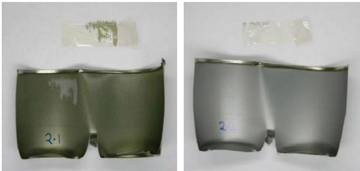
Figure 21: Lacquer adhesion test showing insufficient adhesion (left) and good adhesion (right) (source: Marmann et al., 2011)
