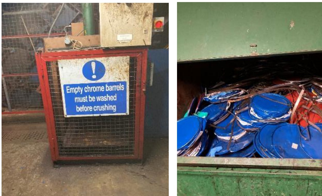
Figure 26: Drum crushing machine (L) and crushed containers (R)
