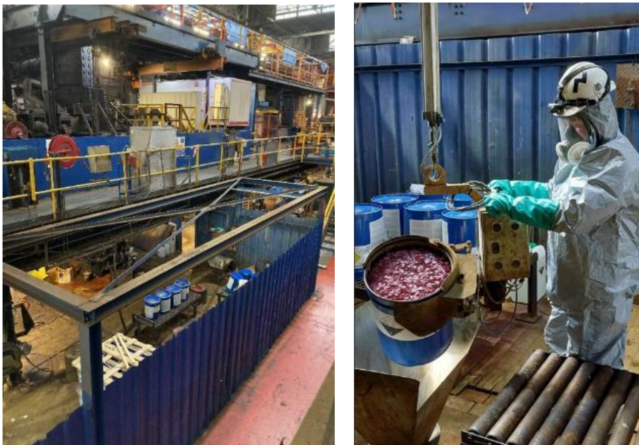
Figure 31: The additions area (L) and lifting of a chromium trioxide container for controlled pouring into the tundish (R)
