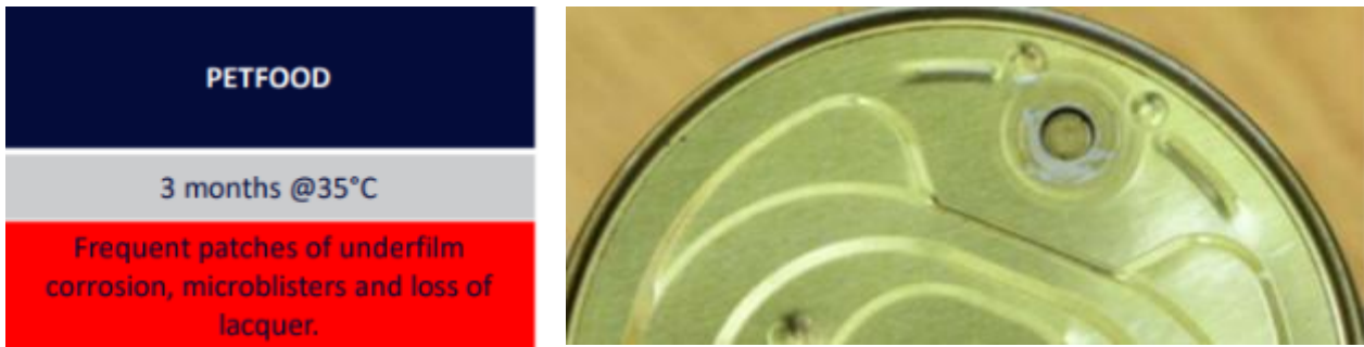
Figure 33: TCCT test results reported after 3 months by Customer A's own customer for fill pack testing
