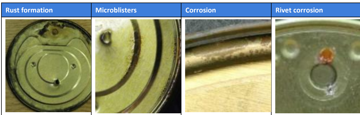
Figure 31: TCCT test results reported after 12 months by Customer A following pack testing of three different coatings at 20°C and 35°C
