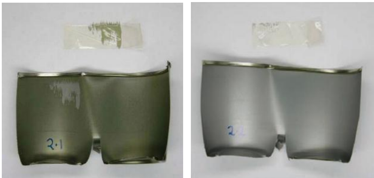
Figure 24: Lacquer adhesion test showing insufficient adhesion (left) and good adhesion (right) (source: Marmann et al., 2011)
