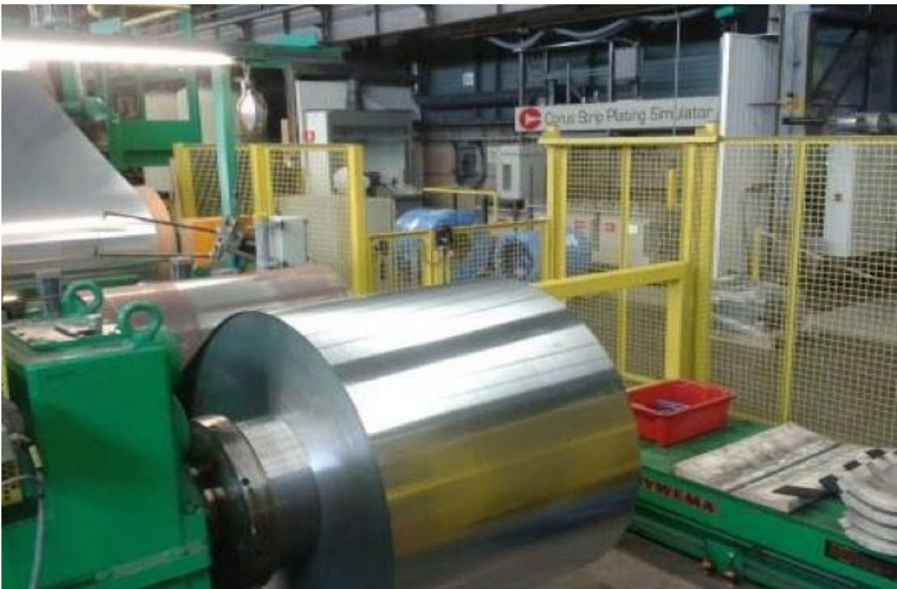
Figure 28: Pilot coating line at IJmuiden for the Cr(III) coating process
